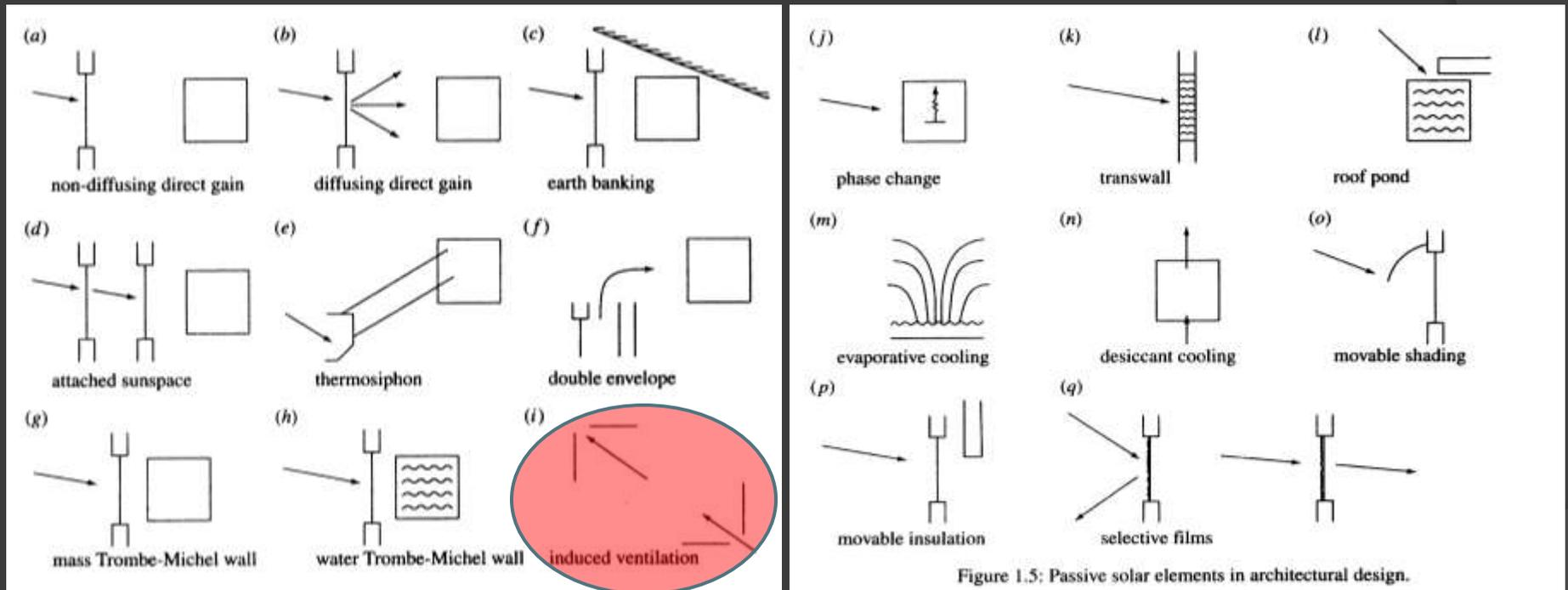
Figure 1.5: Passive solar elements in architectural design.
