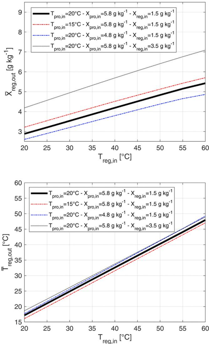
**Fig. 11.** Effect of inlet air conditions on average outlet temperature and humidity ratio of regeneration airflow ( $\tau = 1200$  s;  $L_{bed} = 5.5$  cm;  $v_{pro}^N = v_{reg}^N = 0.5$  m s<sup>-1</sup>; co-current flows).
