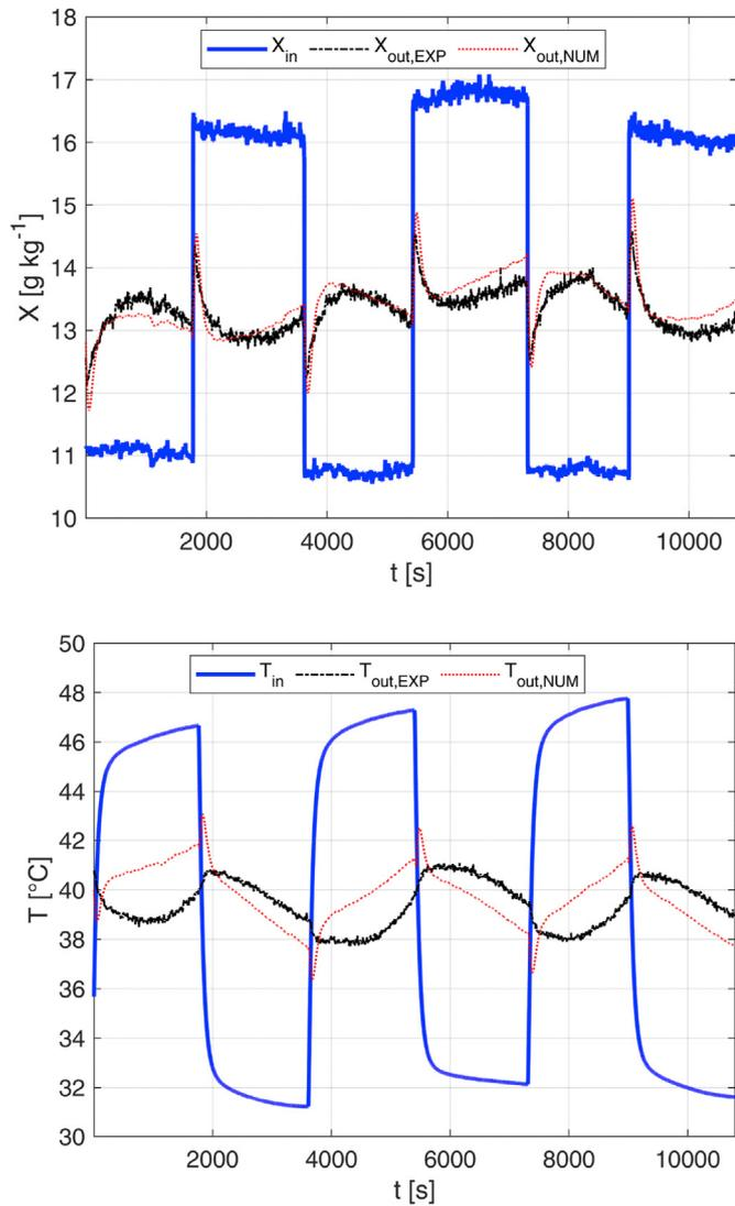
**Fig. 7.** Test 2 - Comparison between experimental data and numerical results: humidity ratio and temperature ( $\tau = 1800$  s;  $v_{pro}^N = 0.56$  m s<sup>-1</sup>;  $v_{reg}^N = 0.56$  m s<sup>-1</sup>;  $L_{bed} = 5.5$  cm).
