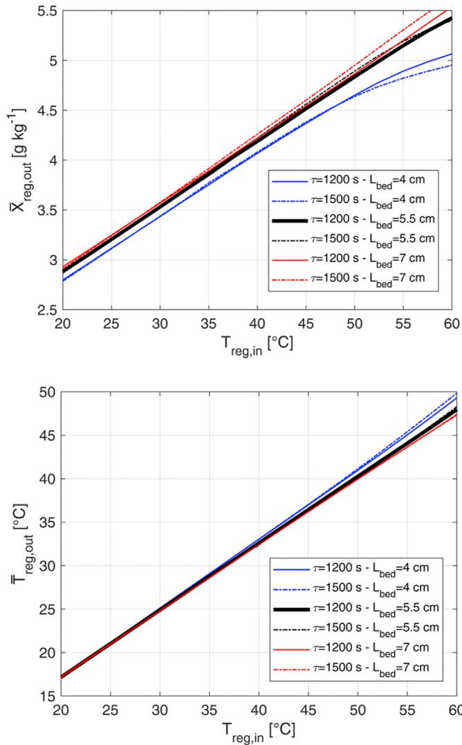
**Fig. 9.** Effect of cycle time and bed length on average outlet temperature and humidity ratio of regeneration airflow ( $v_{pro}^N = v_{reg}^N = 0.5 \text{ m s}^{-1}$ ;  $X_{reg,in} = 1.5 \text{ g kg}^{-1}$ ;  $T_{pro,in} = 20 \text{ }^\circ\text{C}$ ;  $X_{pro,in} = 5.8 \text{ g kg}^{-1}$ ; co-current flows).
