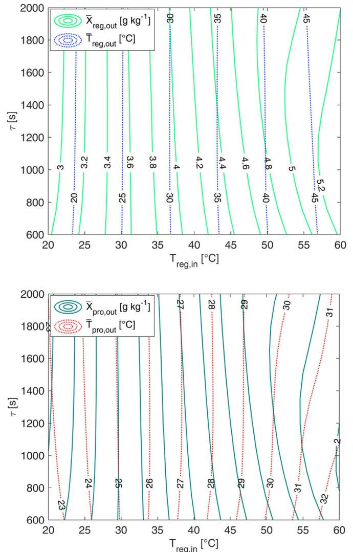
**Fig. 8.** Average outlet temperature and humidity ratio of regeneration and process airflows in the reference configuration ( $v_{pro}^N = v_{reg}^N = 0.5$  m s<sup>-1</sup>;  $L_{bed} = 5.5$  cm;  $X_{reg,in} = 1.5$  g kg<sup>-1</sup>;  $T_{pro,in} = 20$  °C;  $X_{pro,in} = 5.8$  g kg<sup>-1</sup>; co-current flows).
