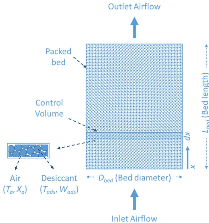
Fig. 2. Scheme of the desiccant beads packed bed.
