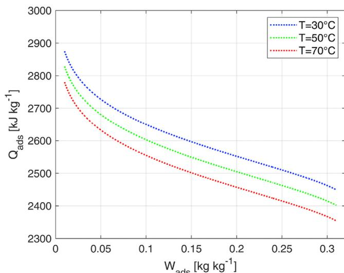
Fig. 4. Calculated heat of adsorption of silica gel (Eq. (22)).
