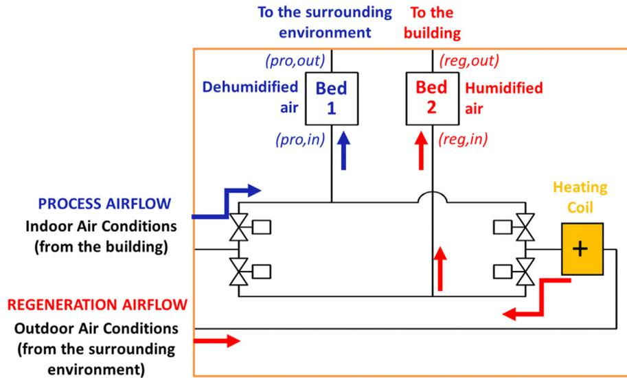
Fig. 1. Working principle of the proposed humidification system.
