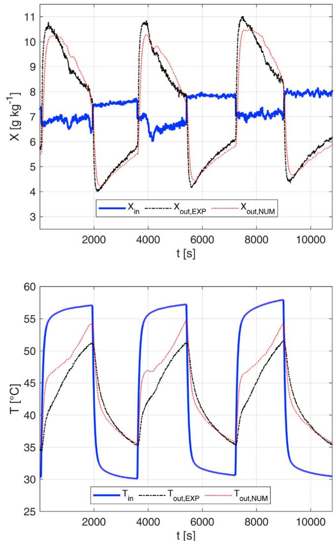
Fig. 6. Test 1 - Comparison between experimental data and numerical results: humidity ratio and temperature ( $\tau = 1800\ s$ ;  $v_{pro}^N = 0.60\ m\ s^{-1}$ ;  $v_{reg}^N = 0.55\ m\ s^{-1}$ ;  $L_{bed} = 5.5\ cm$ ).
