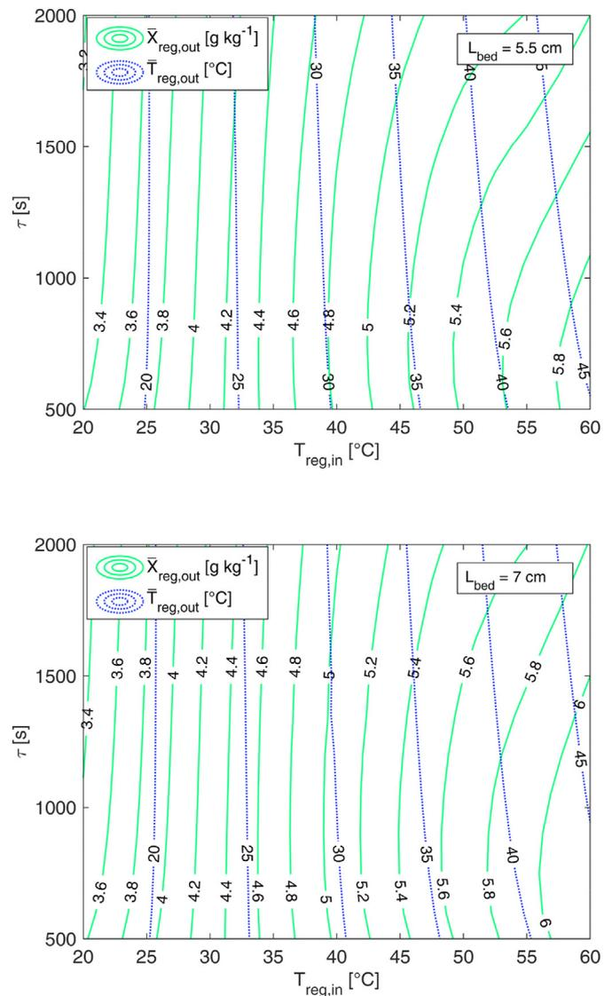
**Fig. 12.** Average outlet temperature and humidity ratio of regeneration airflow in counter-current configuration ( $v_{pro}^N = v_{reg}^N = 0.5$  m s<sup>-1</sup>;  $X_{reg,in} = 1.5$  g kg<sup>-1</sup>;  $T_{pro,in} = 20$  °C;  $X_{pro,in} = 5.8$  g kg<sup>-1</sup>; counter-current flows).
