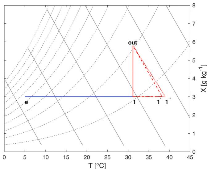
**Fig. 13.** Qualitative representation of humidification process on the psychrometric chart ( $p_{tot} = 101325 \text{ Pa}$ ): i) pre heating (blue solid line); ii) steam humidifier (red solid line); iii) adiabatic humidifier (red dashed line); iv) desiccant humidifier (red dotted line). (For interpretation of the references to colour in this figure legend, the reader is referred to the Web version of this article.)
