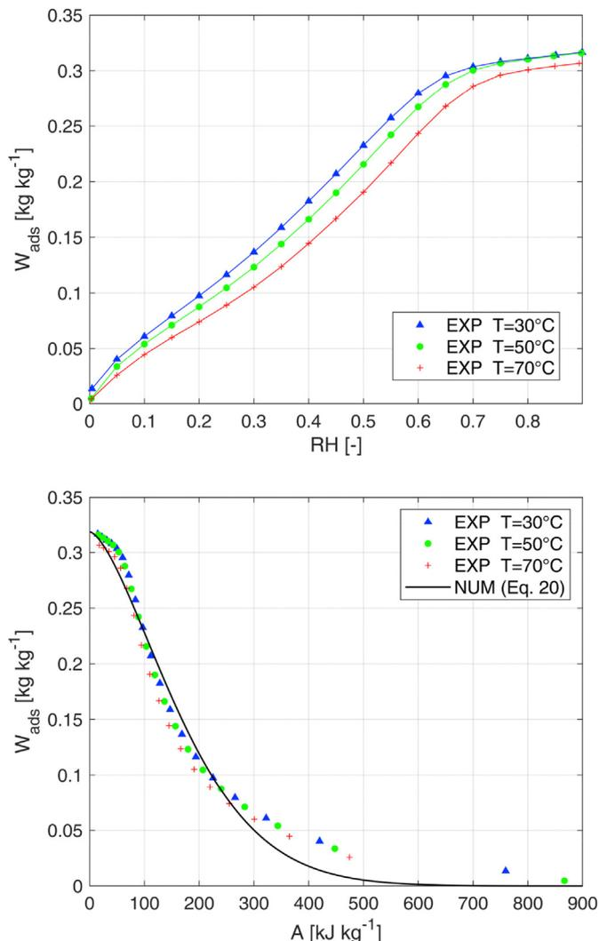
Fig. 3. Measured and calculated equilibrium adsorption capacity of silica gel (numerical results obtained with Eq. (20) and the following parameters:  $W_{ads,max} = 0.3185 \text{ kg kg}^{-1}$ ,  $E = 202.3 \text{ kJ kg}^{-1}$  and  $n = 1.557$ ).
