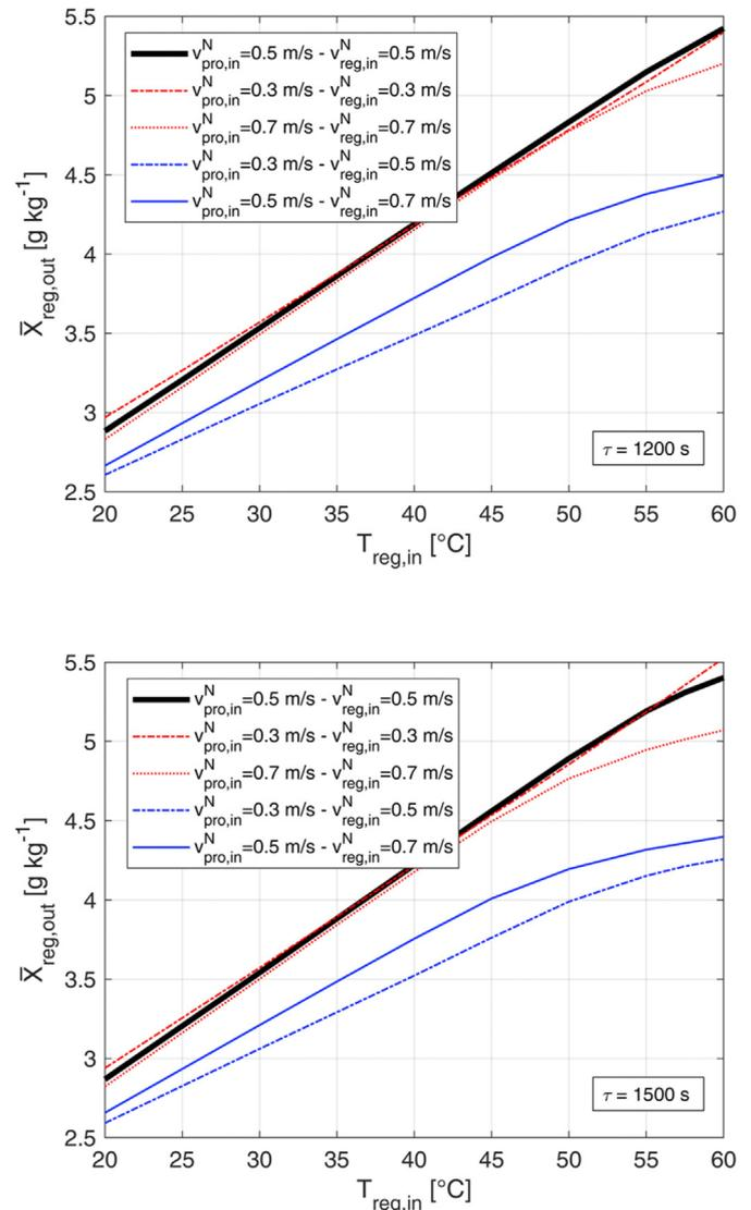
**Fig. 10.** Effect of inlet velocities on average outlet humidity ratio of regeneration airflow ( $L_{bed} = 5.5 \text{ cm}$ ;  $X_{reg,in} = 1.5 \text{ g kg}^{-1}$ ;  $T_{pro,in} = 20 \text{ }^\circ\text{C}$ ;  $X_{pro,in} = 5.8 \text{ g kg}^{-1}$ ; co-current flows).
