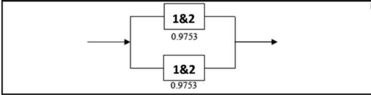
**Fig. 5.9** Block diagram illustration of reliability of components installed in parallel
