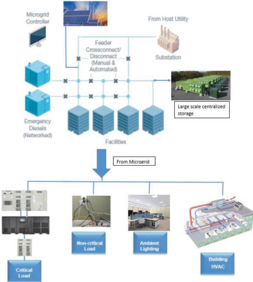
**Fig. F.18** Microgrid with centralized emergency generators, RE sources, and a centralized storage
