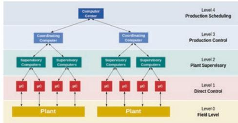
Fig. F.77 Control center Energinet.dk and SCADA structure
