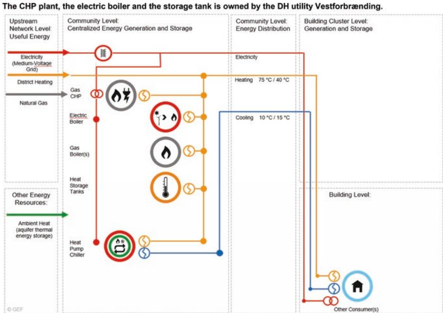
**Fig. 7.16** Smart energy system at the campus of the Technical University of Denmark in Lyngby
