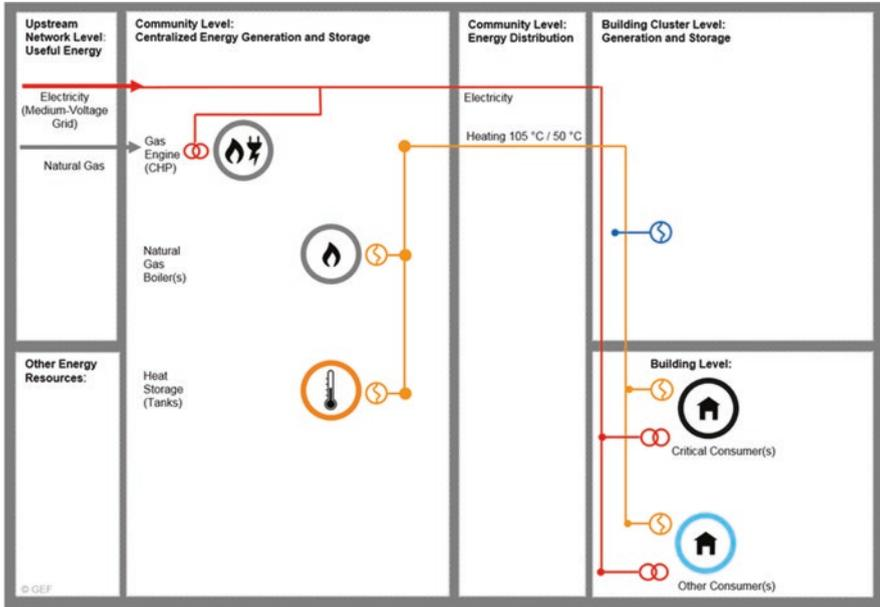
Fig. E.1 Thermal energy system architecture
