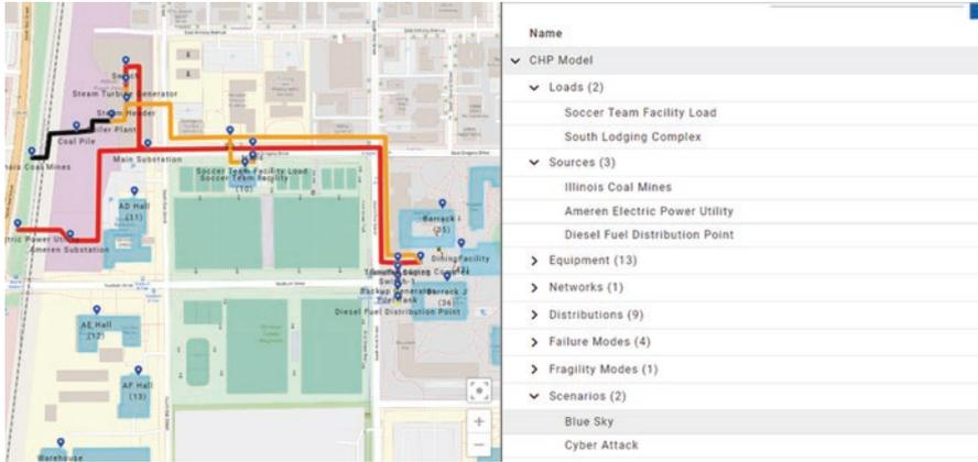
**Fig. 8.14** The above figure shows the system as modeled in the integrated SMPL/ERIN system. ERIN components and buildings are represented by blue icons. Utilities such as the CHP plant and commercial grid are on the left of the map, the Soccer Team Facility is at the center, and the South Lodging complex is to the right. The right-hand pane shows a tree of the components of the ERIN model
