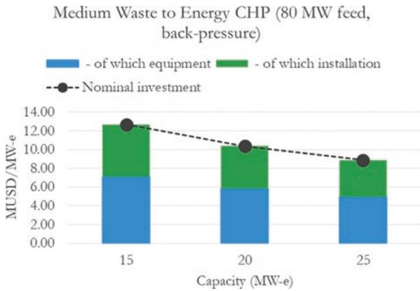
**Fig. F.13** Nominal investment for a medium waste-to-energy CHP (80 MW feed, back-pressure)
