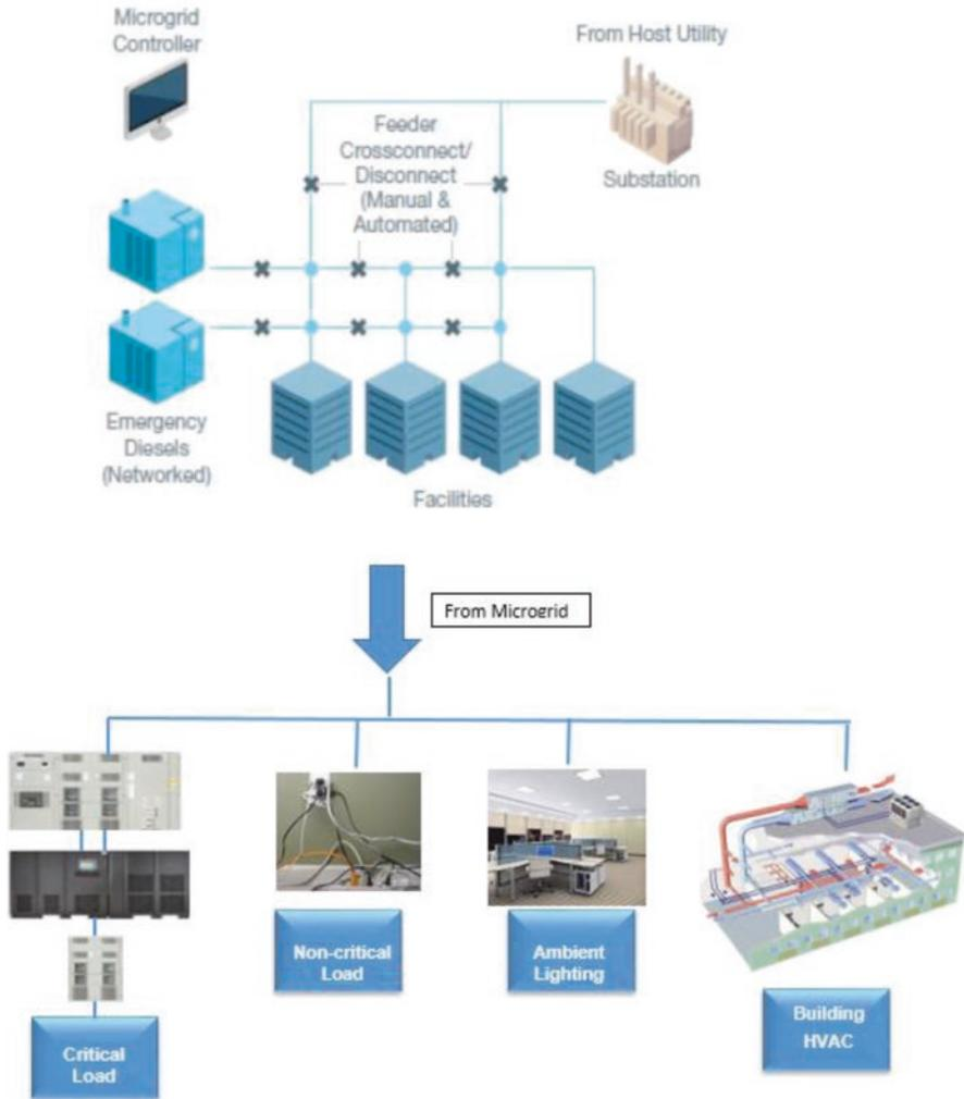
Fig. F.19 Microgrid with centralized emergency generators
