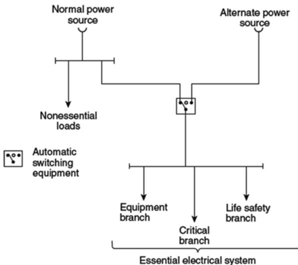
Fig. C.9 Example of a hospital one-line traditional diagram. (Courtesy NFPA 70 [2020])
