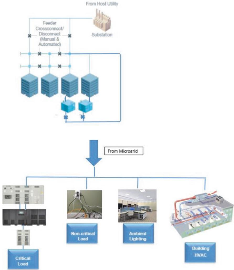
Fig. F.21 Microgrid with decentralized emergency generators
