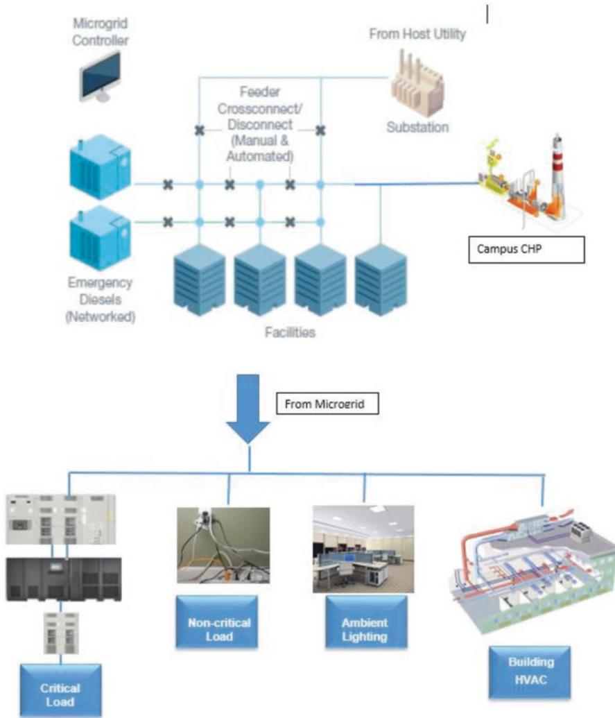
Fig. F.17 Microgrid with centralized emergency generators and CHP plant
