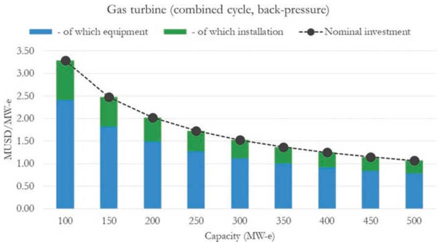
**Fig. F.5** Nominal investment for gas turbine (combined cycle, back-pressure)
