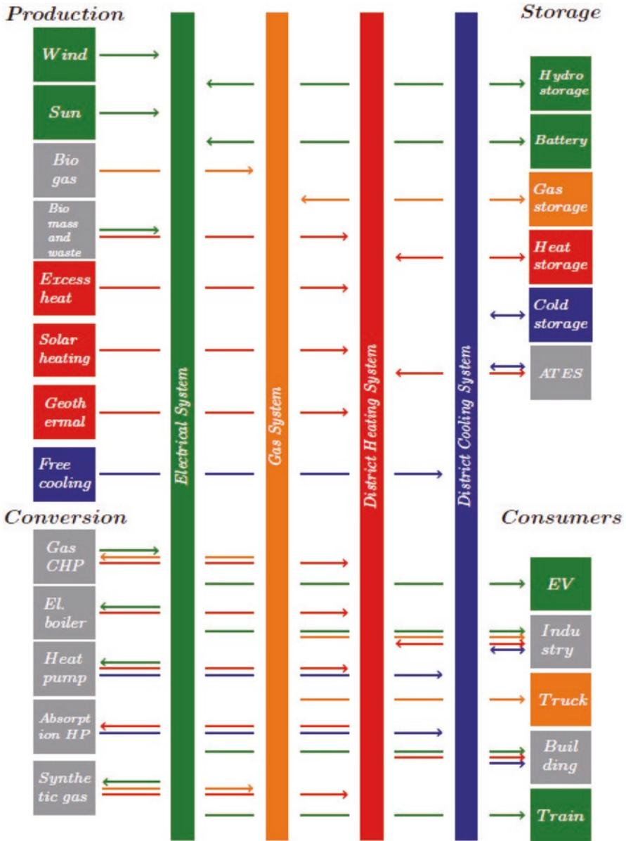
Fig. 7.7 The integrated energy system with four energy carriers
