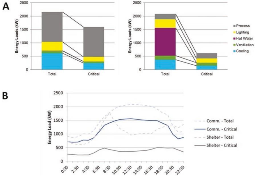
**Fig. 3.6** Total and critical electrical demands: (a) total and critical electrical demand load for a data center (left) and a dormitory (right) and (b) critical electrical demand hourly profiles for communications and shelter over a 24-h period
