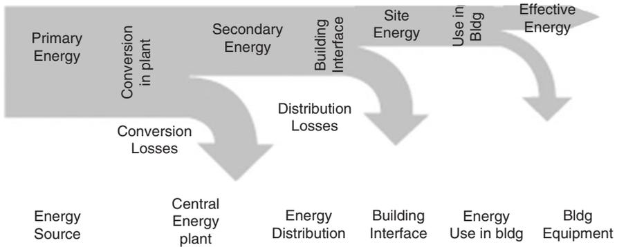
**Fig. 3.5** Energy supply chain from primary energy to its use inside a building. (Zhivov et al. 2015)
