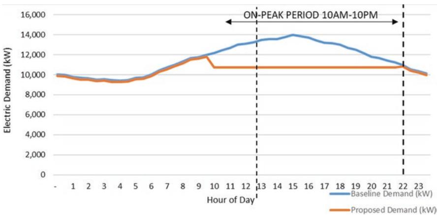
**Fig. I.2** During a peak shaving event, the demand, as seen by the utility, is actively managed by the DERs
