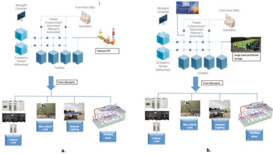
**Fig. 7.11** (a) Microgrid with centralized emergency generators and CHP plant; (b) microgrid with centralized emergency generators, RE sources, and centralized storage
