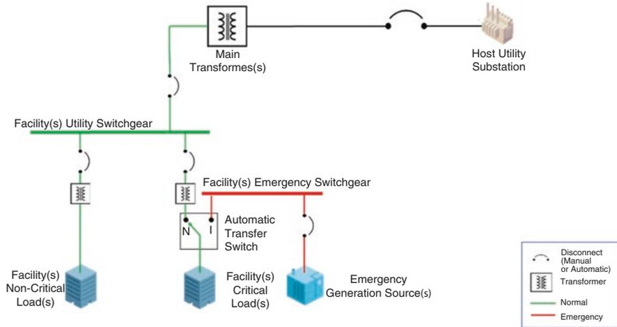
Fig. 7.9 Emergency generator serving mission-critical facility load
