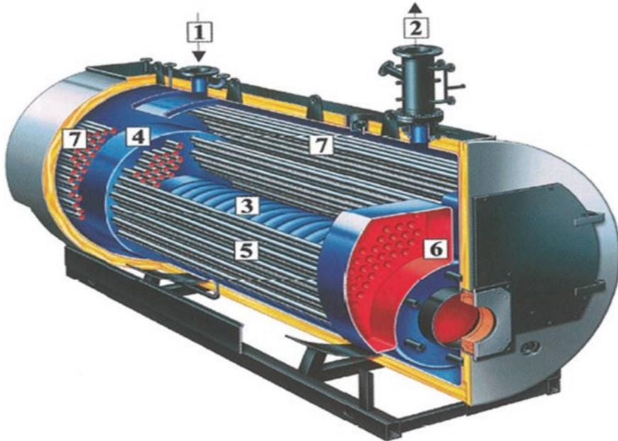
**Fig. F.35** Natural gas boiler
