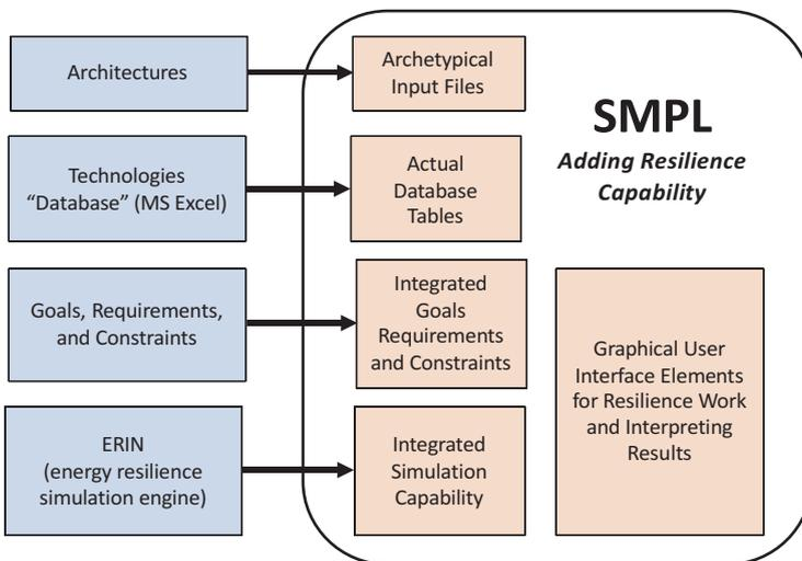
**Fig. 8.12** Integration of IEA Annex 73/EW18-5281 technology into the SMPL tool. Currently, the ERIN engine and parts of the technologies database have been integrated into SMPL. Architectures, goals, requirements, and constraints require future work
