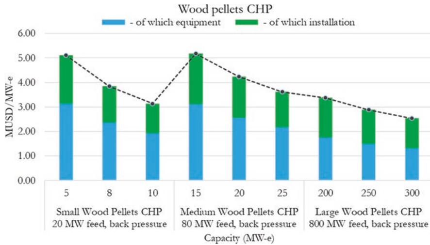
Fig. F.10 Nominal investment for wood pellets CHP (20, 80, 800 MW feed, back-pressure)
