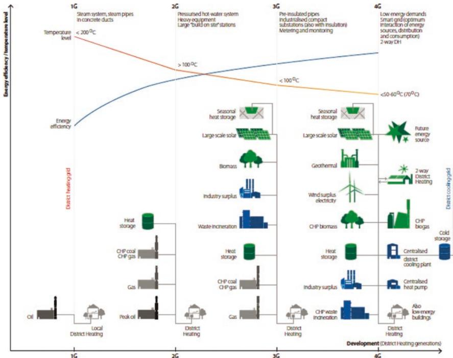
Fig. 7.1 Four generations of thermal district systems. (Reproduced with permission from [www.4dh.dk](http://www.4dh.dk))
