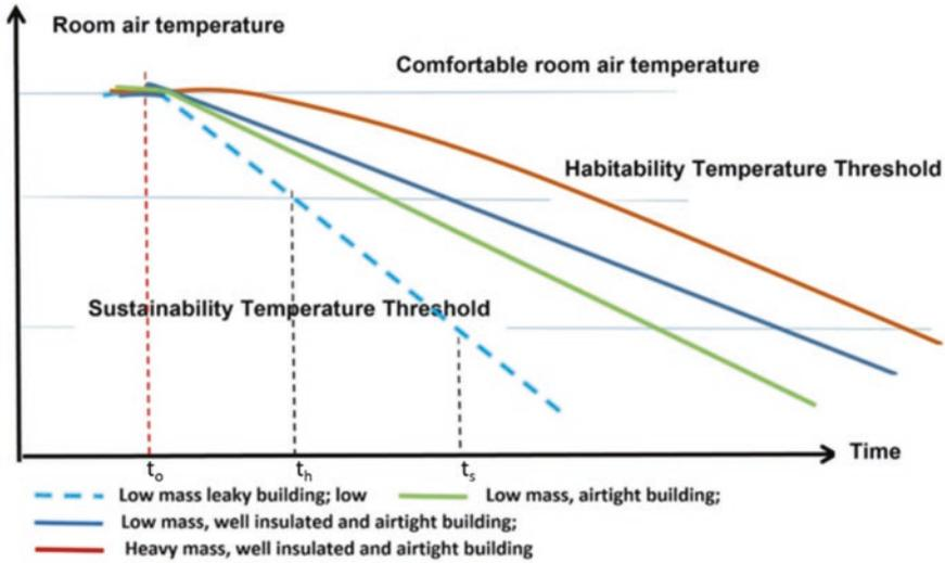
Fig. 5.16 Notional example of temperature decay rate for different types of building envelope
