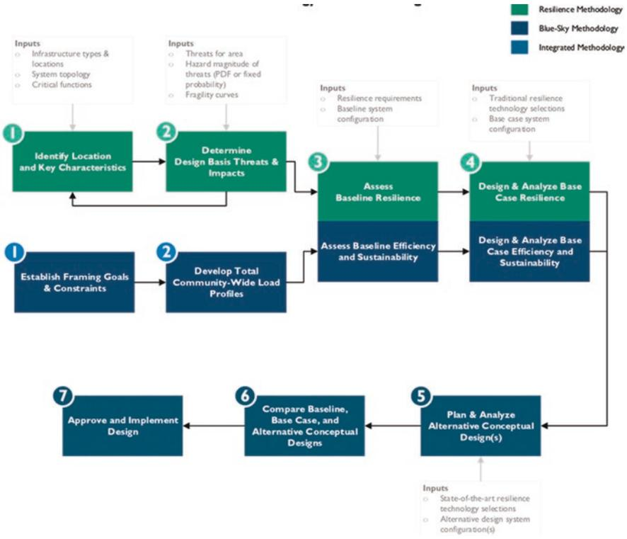
Fig. ES.1 Integration of energy systems resilience analysis into energy master plan
