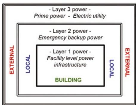
that resides inside the facility. Common components are an uninterruptible power supply (UPS) and an automatic transfer switch (ATS). Layer one backup power is the shortest duration of electrical power capacity of the three layers. The power delivery capacity can typically be from several minutes to several hours.
