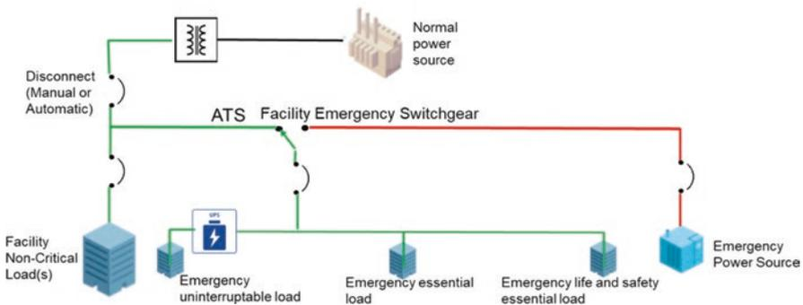
Fig. C.1 Schematic of the one-line diagram for a notional facility
