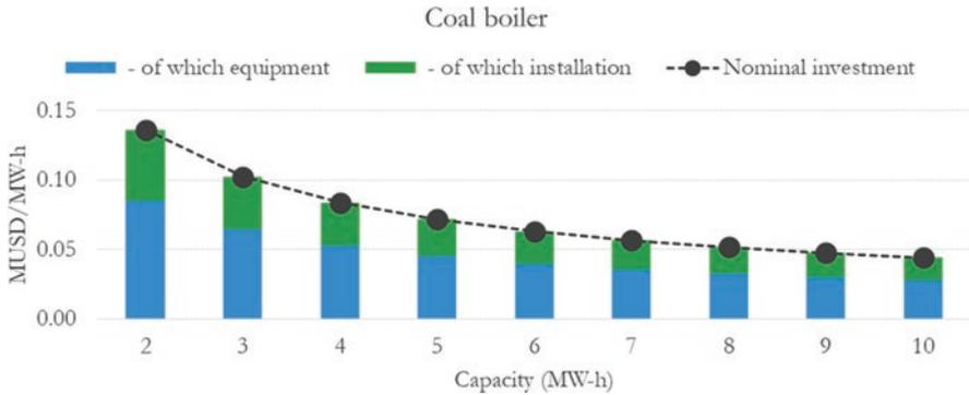
**Fig. F.43** Nominal investment by capacity for a coal boiler
