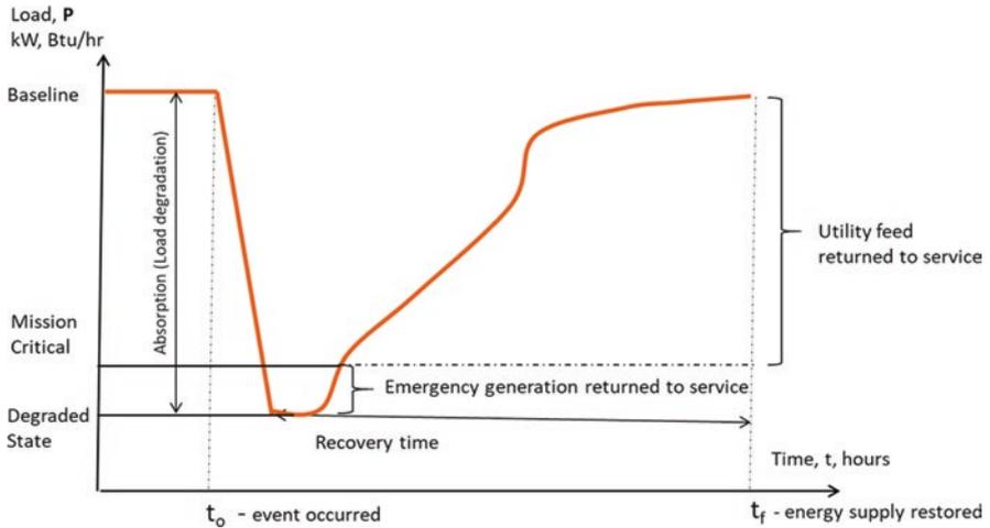
Fig. 5.6 Stepped recovery of power system assets
