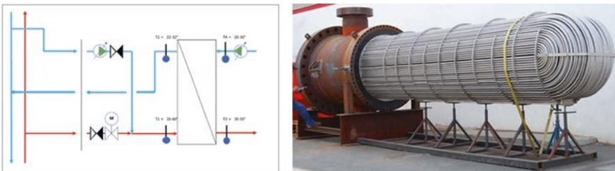
**Fig. F.73** Heat exchanger station and bundle-type heat exchanger
