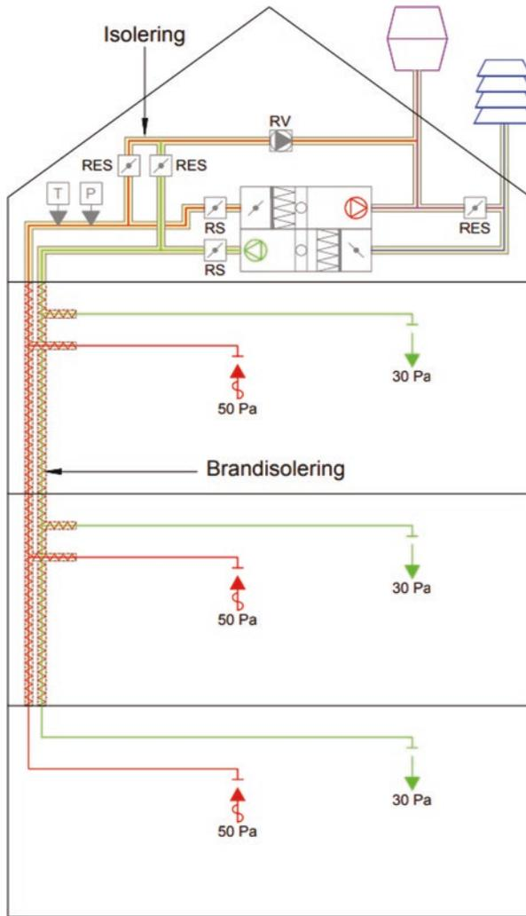
Fig. F.70 Central ventilation with heat recovery
