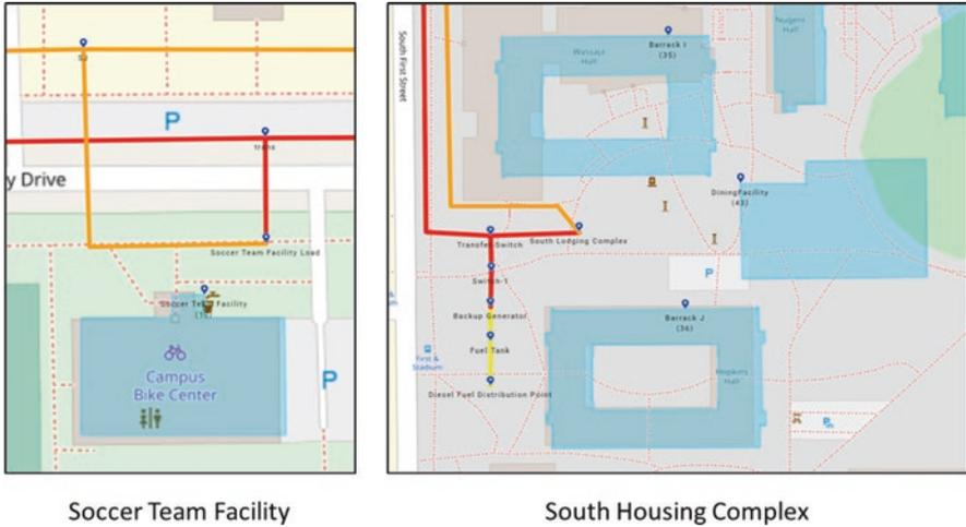
**Fig. 8.15** Energy loads in ERIN are modeled by load components. SMPL enables creation of load components and association of SMPL building energy models with those components. When an ERIN simulation is run, SMPL creates energy load profiles for ERIN. If multiple buildings are associated with a load, then SMPL will aggregate the loads prior to creating the load files
