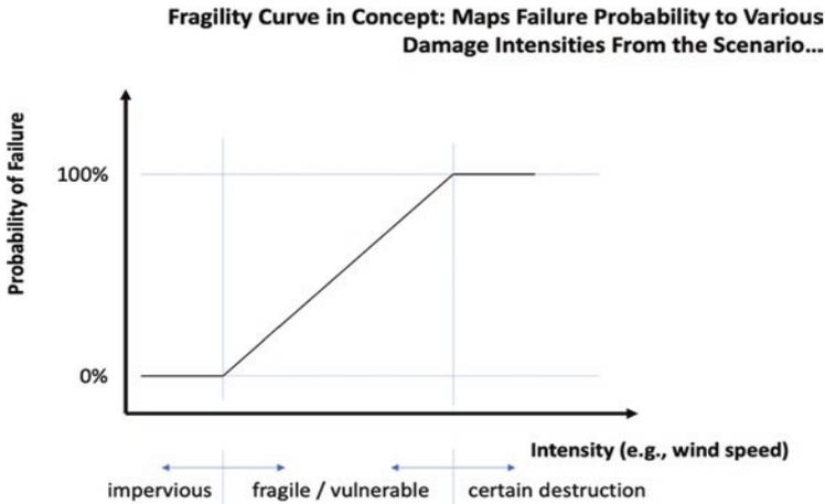
**Fig. 8.4** Example fragility curve using impervious and certain destruction information
