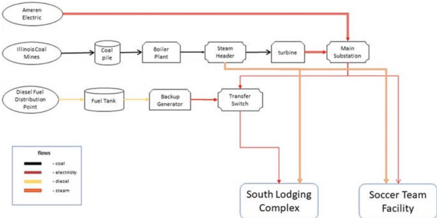
**Fig. 8.13** Schematic of a system to be modeled in the ERIN/SMPL integrated tool. Notice that the CHP plant generates both electricity and steam, with additional electricity coming from the commercial grid. The Soccer Team Facility represents a typical energy load with no backup, while the South Lodging Complex represents a “critical” load and thus has a backup generator. Note that there is no backup for the steam beyond redundancy within the boiler plant
