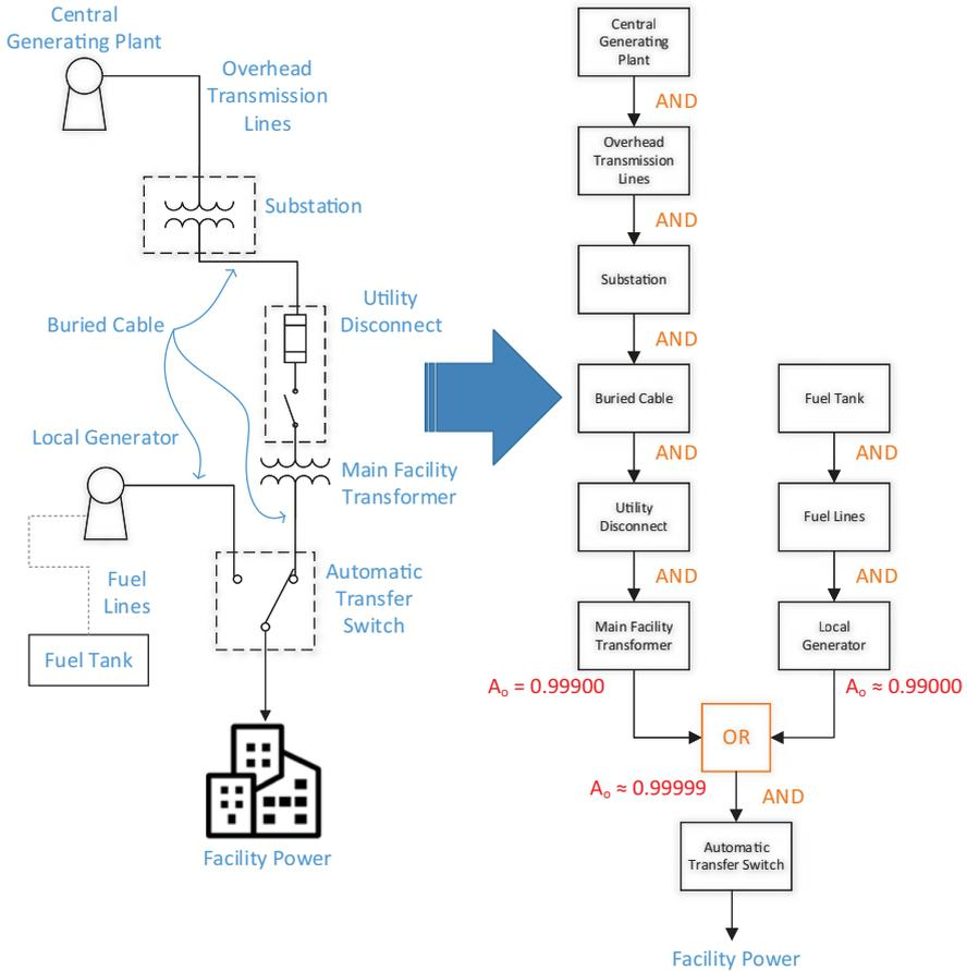
Fig. 5.10 Reliability block diagram for a typical distribution system
