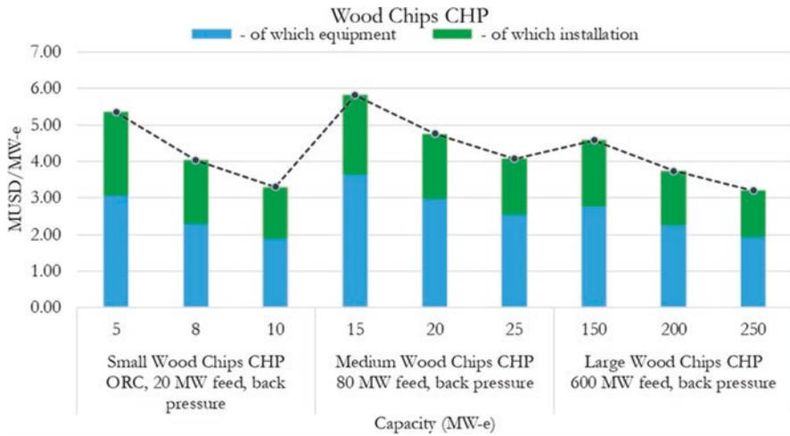
Fig. F.9 Nominal investment for a wood chips CHP (20, 80, 600 MW feed, back-pressure)
