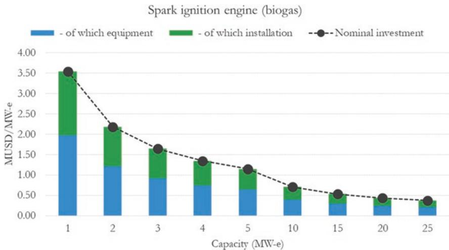
Fig. F.3 Nominal investment by capacity for a spark ignition engine using biogas
