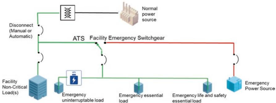
**Fig. 5.1** Schematic of the one-line diagram for a notional facility
