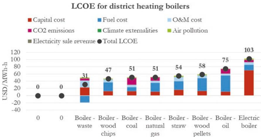
Fig. F.34 LCOE for district heating boilers
