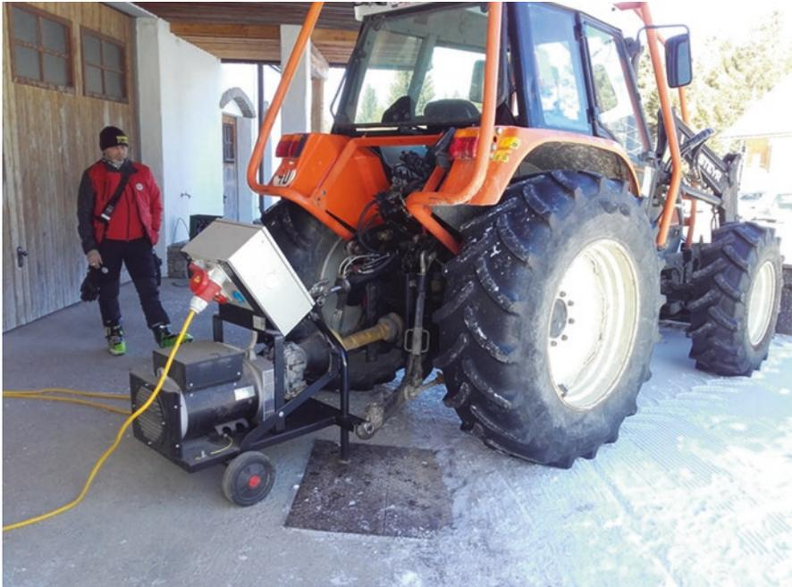
**Fig. B.7** Tractor providing power to a mountain resort during 3-hour blackout. This is a typical mobile backup method used in agricultural and sparsely populated areas (February 2020, Sommeralm in Austria. Source: AEE INTEC)
