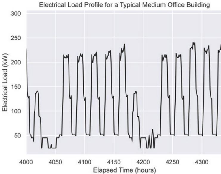
**Fig. 8.5** Load profile for a typical medium office building in Palmdale, CA
