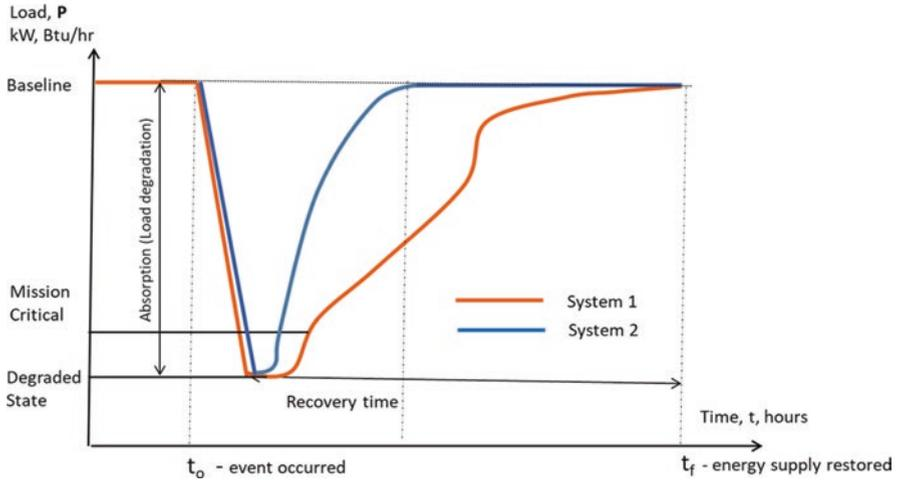
**Fig. 5.5** Two systems with different recovery times
