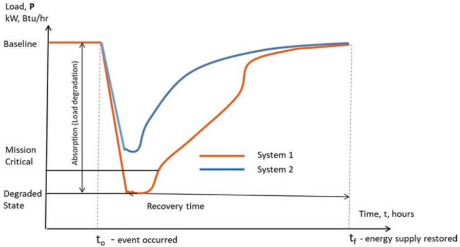
Fig. 5.4 Two systems with different absorption
