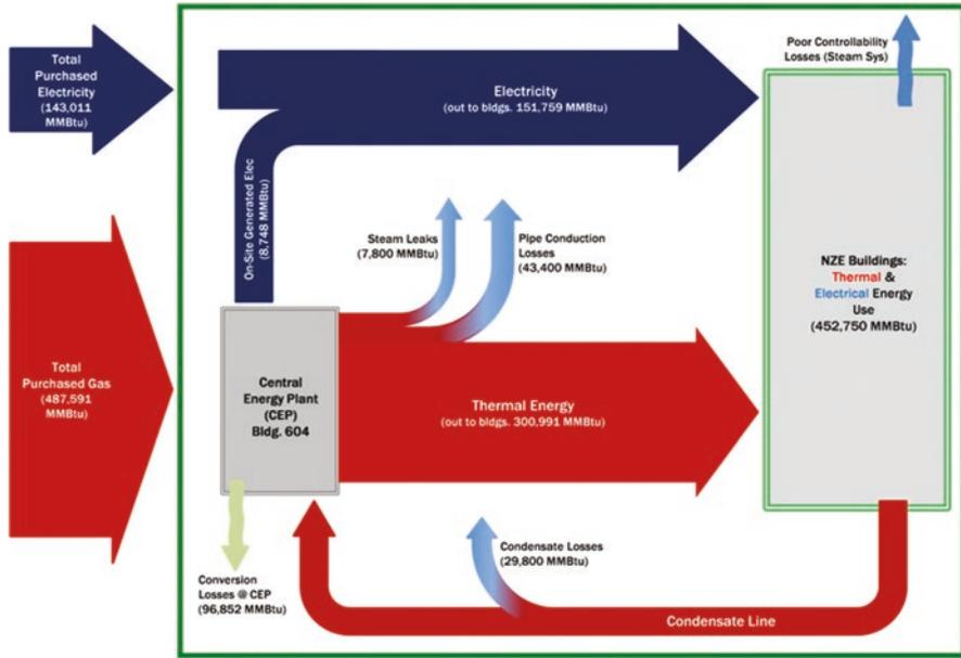
**Fig. 3.4** Schematic of Baseline energy uses and wastes at a net-zero energy (NZE) area of one military installation. (Zhivov et al. 2015)
