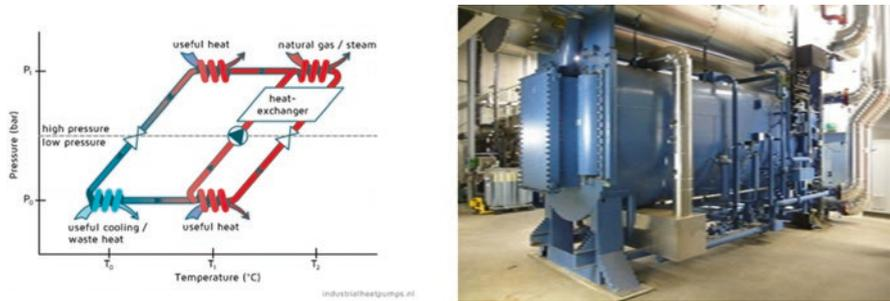
**Fig. F.46** Absorption heat pump
