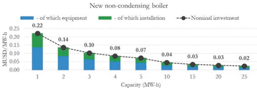
**Fig. F.37** Nominal investment by capacity of new non-condensing natural gas boiler
