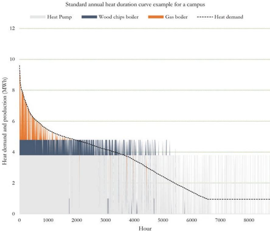
**Fig. 7.8** Standard annual heat duration curve example for a campus simulated with EnergyPro. (Provided by Ramboll)
