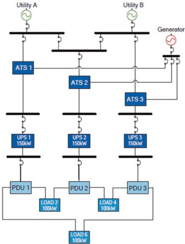
Fig. C.7 Tri-redundant UPS configuration (no STS). (McCarthy and Avelar 2016)
