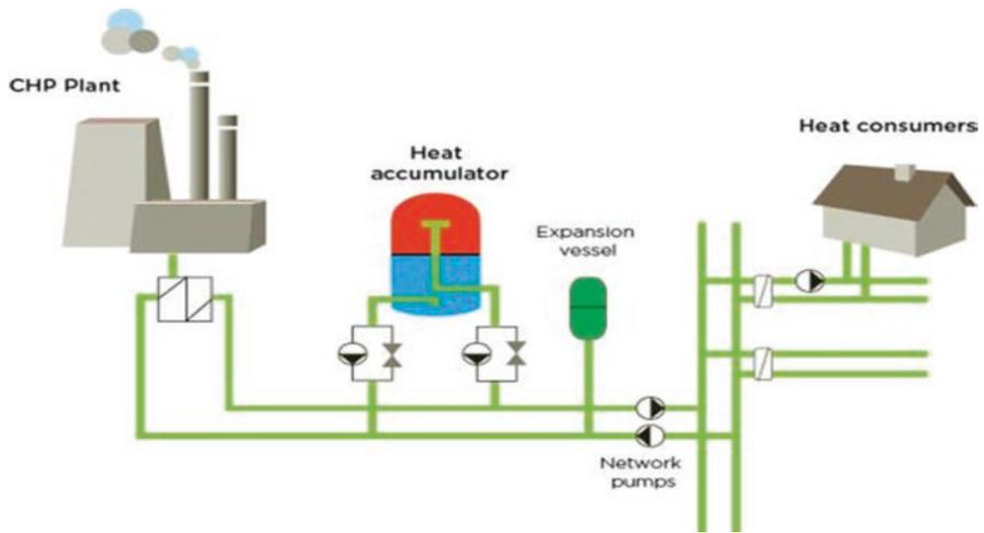
**Fig. F.53** This tank is sectioned from the pressure in the network. The operator has to start and stop loading and unloading
