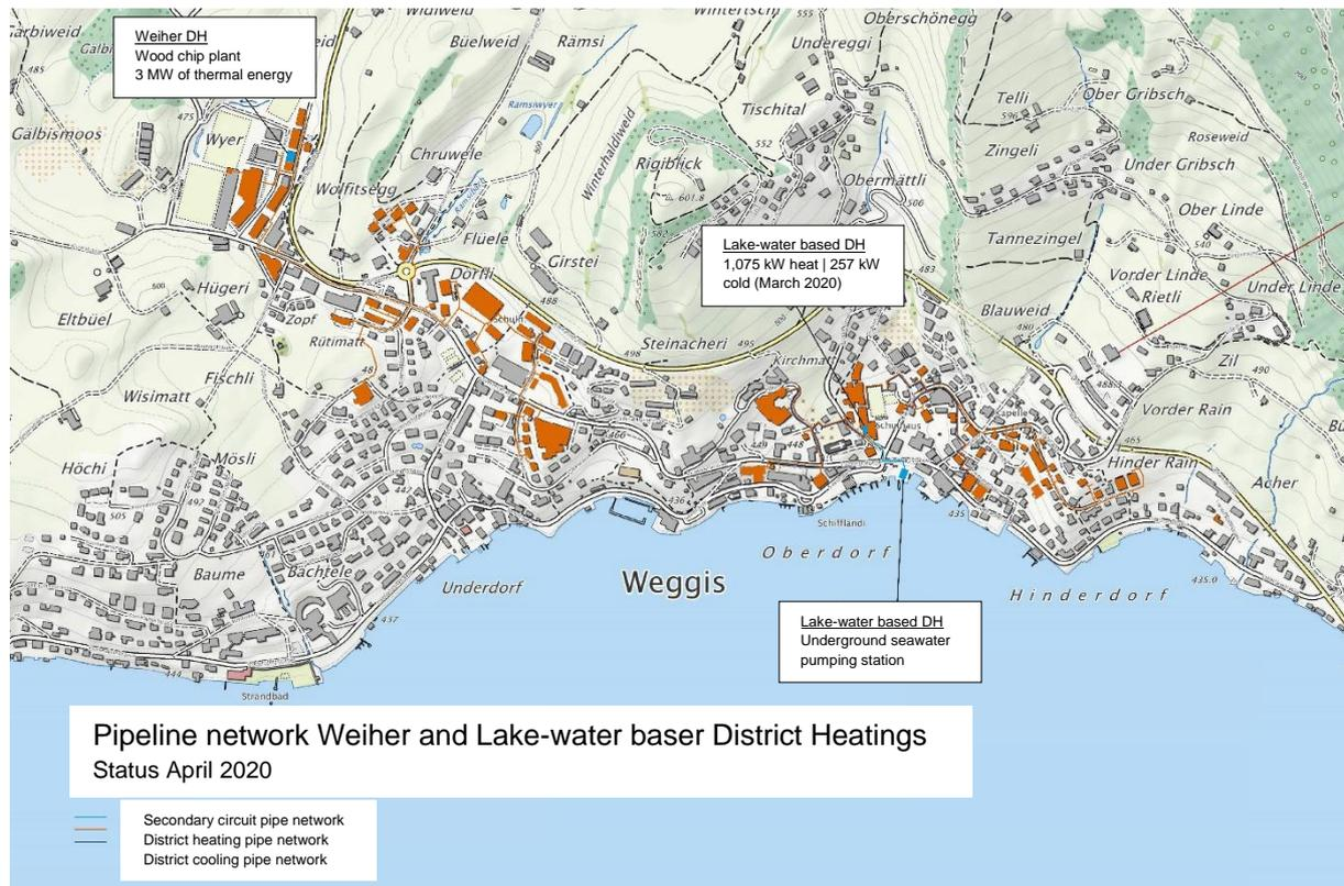
Figure 2. Schematic view of the buildings connected in April 2020 and of the existing pipeline network (Source: Corporation Weggis).
