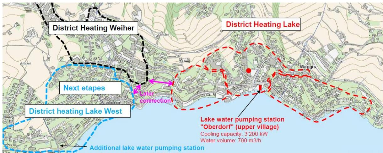
Figure 1. Schematic view of the different stages of the district heating networks in Weggis (Source: Corporation Weggis).
