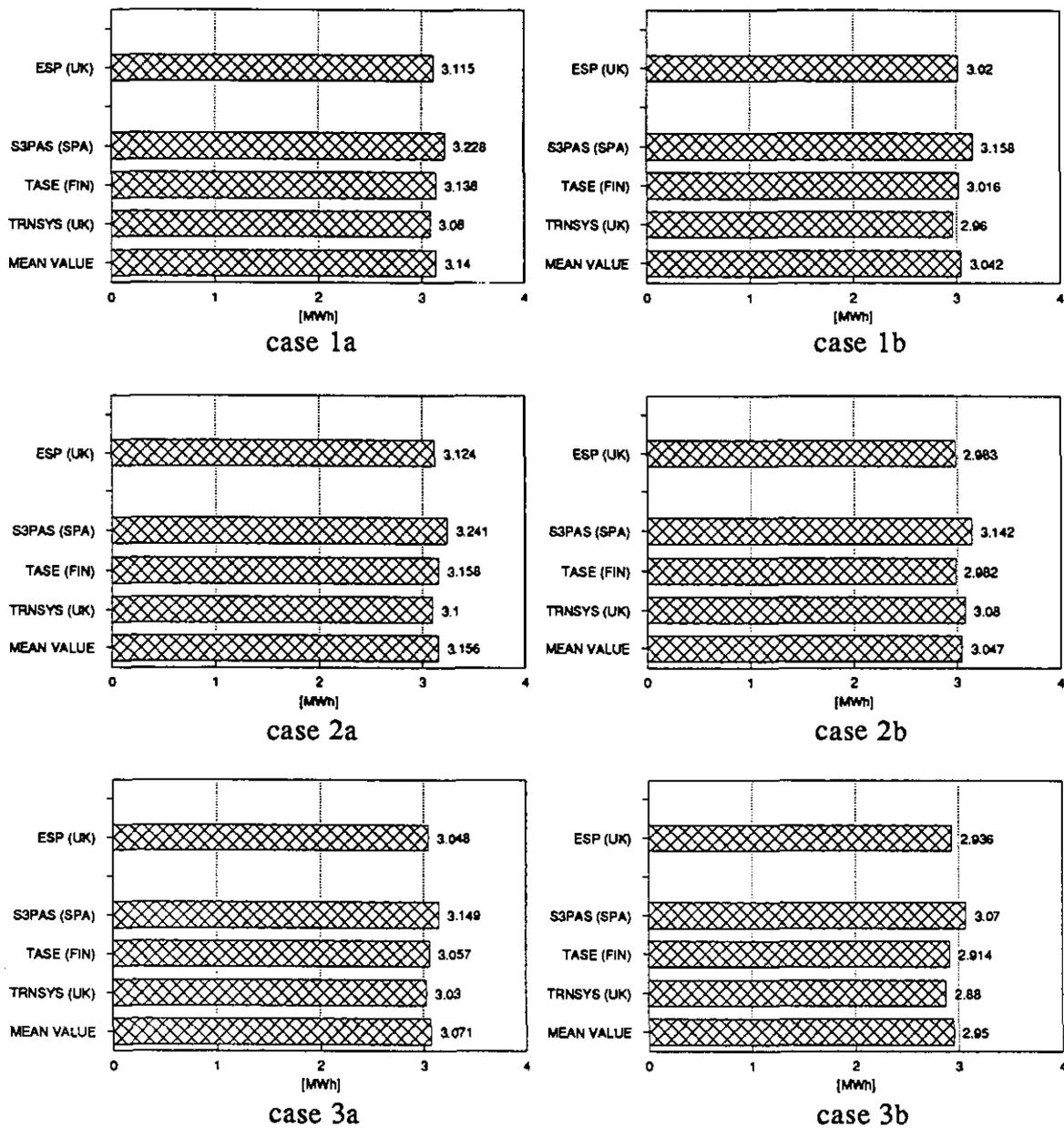
Figure 15. Annual heat losses of ventilation of the whole module.
