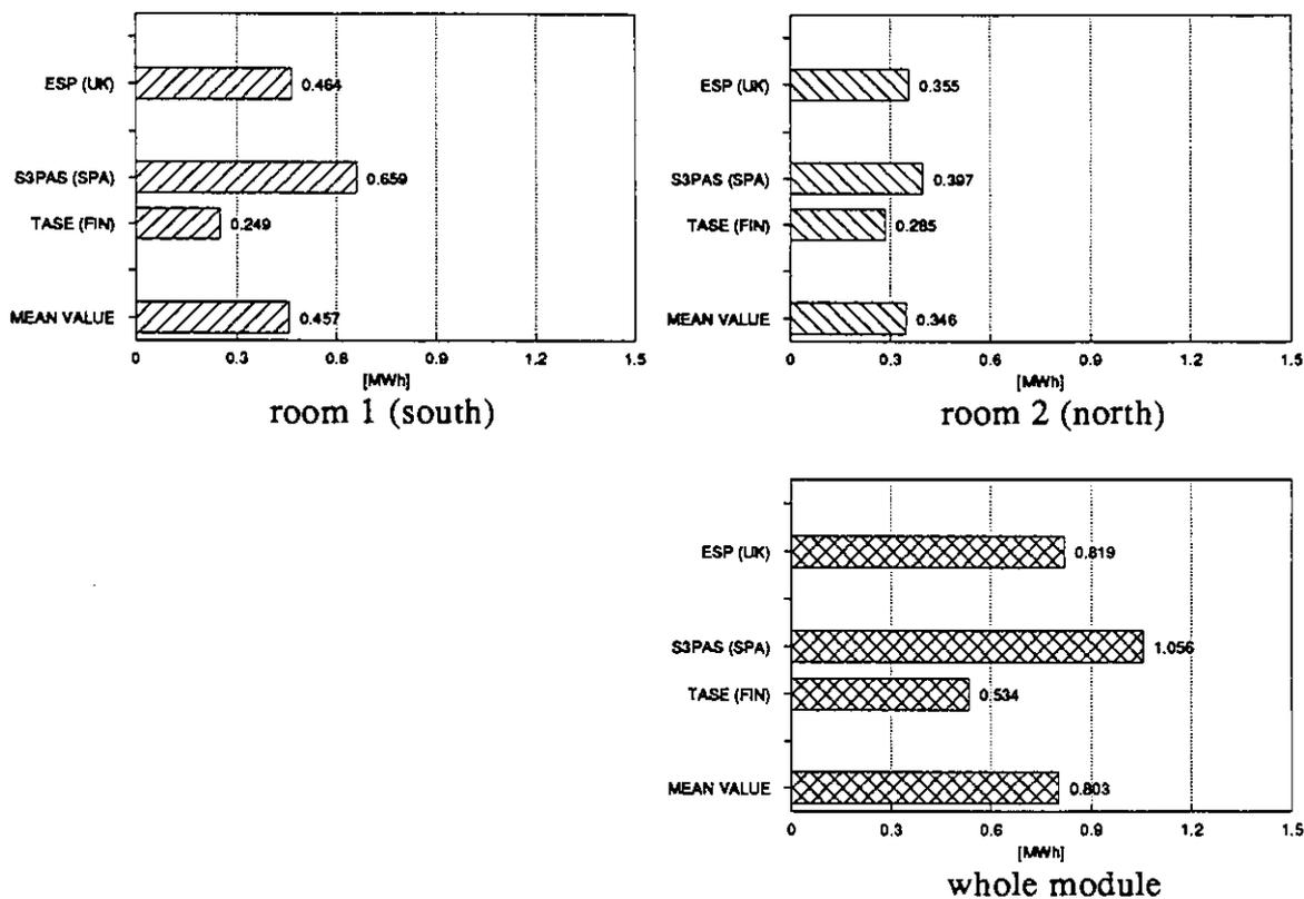
Figure 13.3a Annual heat losses through exterior walls in case 3a.
