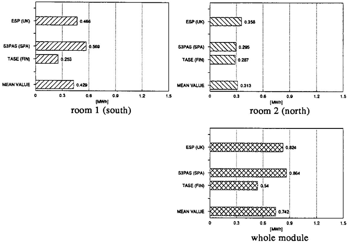
Figure 13.1a Annual heat losses through exterior walls in case 1a.
