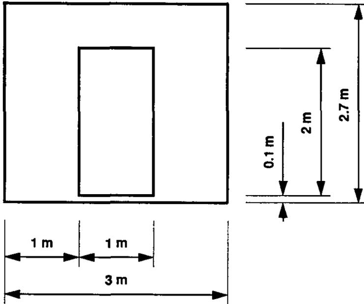
Figure 3. Dimensions of internal wall with door.
