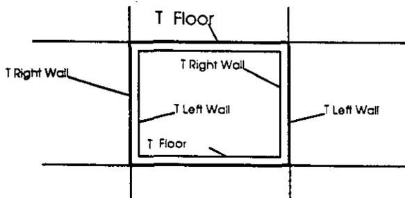
Figure 2 - Modelling adjacent zones with identical conditions in TRNSYS. The surface temperature used for the other side of separating fabric elements are assumed to be equal to that of the inside surface of their opposite elements.
