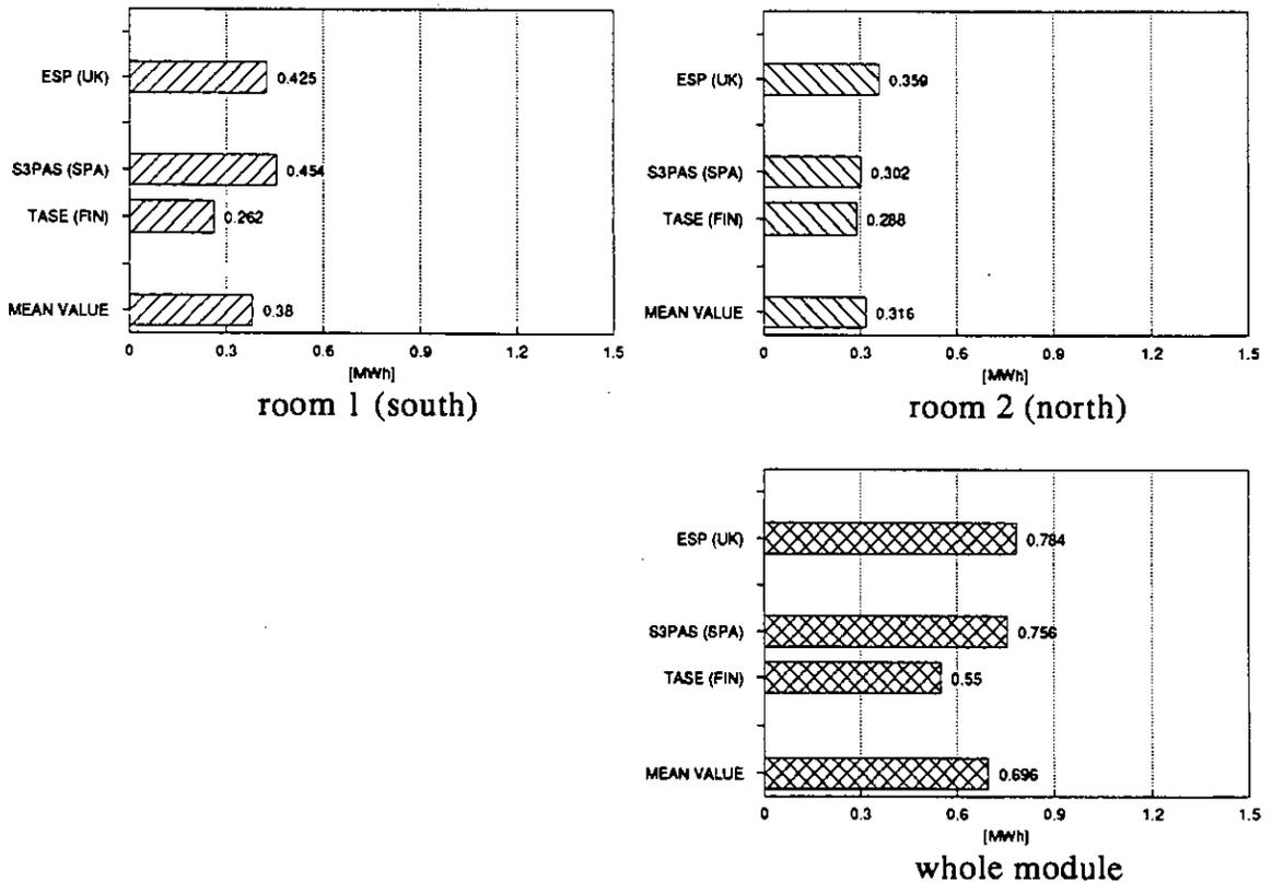
Figure 13.1b Annual heat losses through exterior walls in case 1b.
