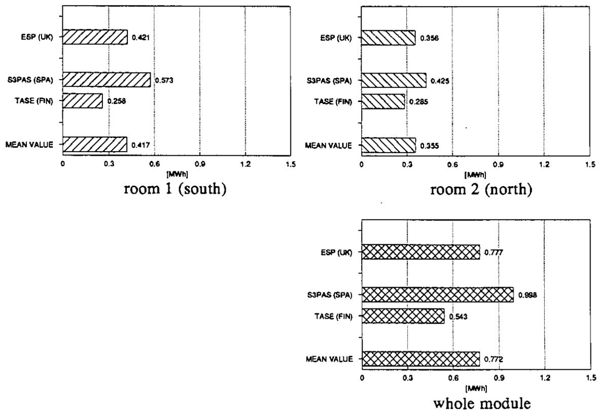
Figure 13.3b Annual heat losses through exterior walls in case 3b.
