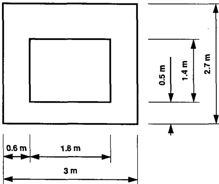
Figure 4. Dimensions of external wall with window.
