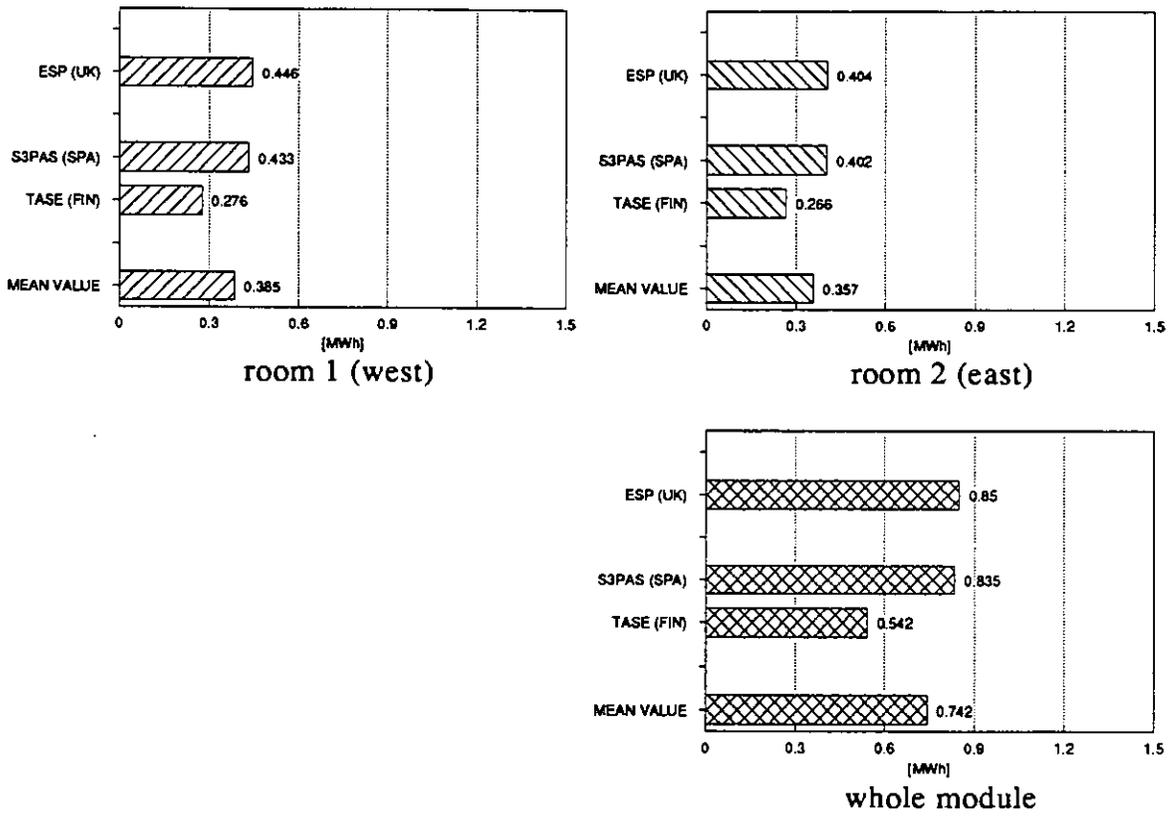
Figure 13.2a Annual heat losses through exterior walls in case 2a.
