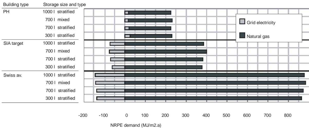
Fig. 38 Influence of storage size on NRPE demand for the SFH building types equipped with SOFC system, for moderate DHW demand profile and UCTE mix.
