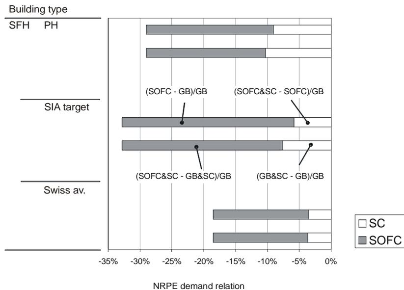
Fig. 28 Comparison of different systems without and with solar collectors (“& SC”), expressed as percentage ratio of NRPE demand of the system, related to the demand standard gas boiler system without solar collector (GB). SFH buildings. UCTE electricity mix.
