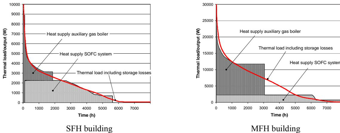
Fig. 31 Thermal load and heat output duration curves for the SOFC system and the SFH (left) and MFH (right) SIA building type
