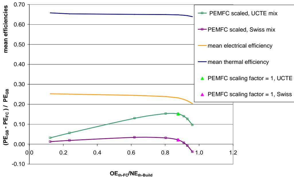
Fig. 37 Difference between NRPE demand of PEMFC cogen system equipped building  $PE_{PEMFC}$  and NRPE demand of reference building with gas boiler system  $PE_{GB}$ , weighted with  $PE_{PEMFC}$ , as a function of ratio of specific annual thermal output of fuel cell cogen unit ( $OE_{th-Fc}$ ) to total annual heat demand of building ( $NE_{th-Build}$ ), for UCTE and Swiss electricity mix. Also shown are the mean electrical and thermal efficiencies.
