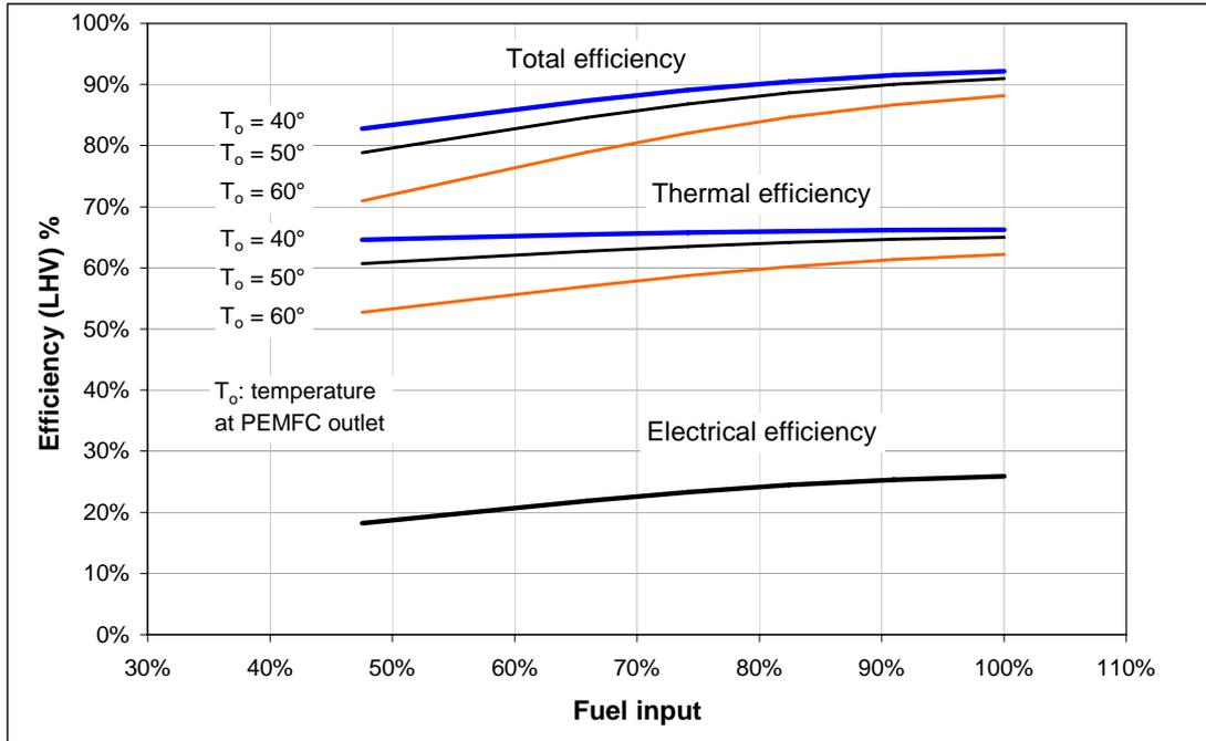
Fig. 8 Electrical (AC to grid), thermal and total efficiency performance characteristics of the 4.6 kWe PEMFC unit considered, in relation to the power input of the fuel (lower heating value), for three different levels of outlet/supply flow temperatures
