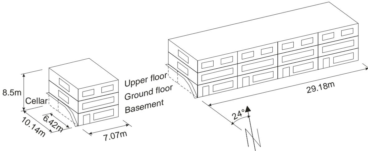
Fig. 5 Geometry and orientation of SFH building (left) and MFH building (right).
