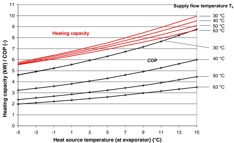
Fig. 12 Heating power capacity and COP curves of the considered heat pump, in function of the heat source temperatures (at entry to evaporator, for different levels of heat supply temperatures ( $T_s$ ))
