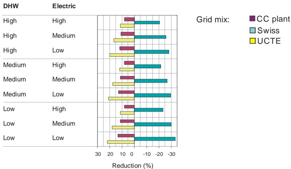
Fig. 43 Relative  $CO_2$ -eq emission reductions for the SHF SIA target building equipped with SOFC system compared to the gas boiler grid reference system, for different DHW and electric demand levels, and for the 3 electricity mixes.
