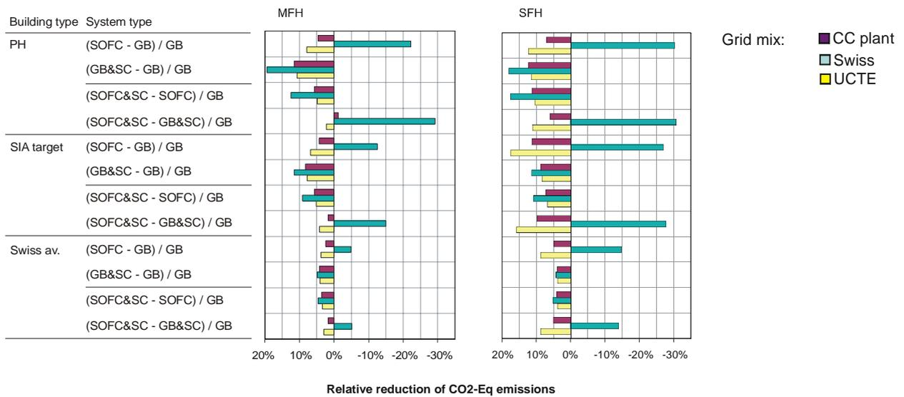
Fig. 30 Comparison of different systems without and with solar collectors (“& SC”) in terms of annual CO<sub>2</sub>-eq emissions, expressed as percentage of CO<sub>2</sub>-eq emission reduction in relation to standard gas boiler system without solar collector (GB), for the three electricity generation mixes
