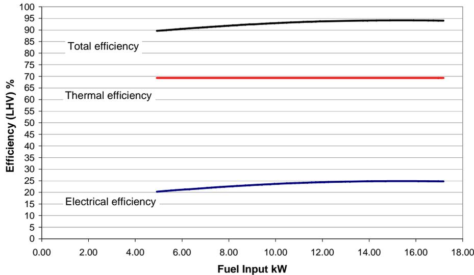
Fig. 10 Electrical, thermal and total efficiency performance characteristics of the 4.7 kWe ICE1 unit considered for SFH.
