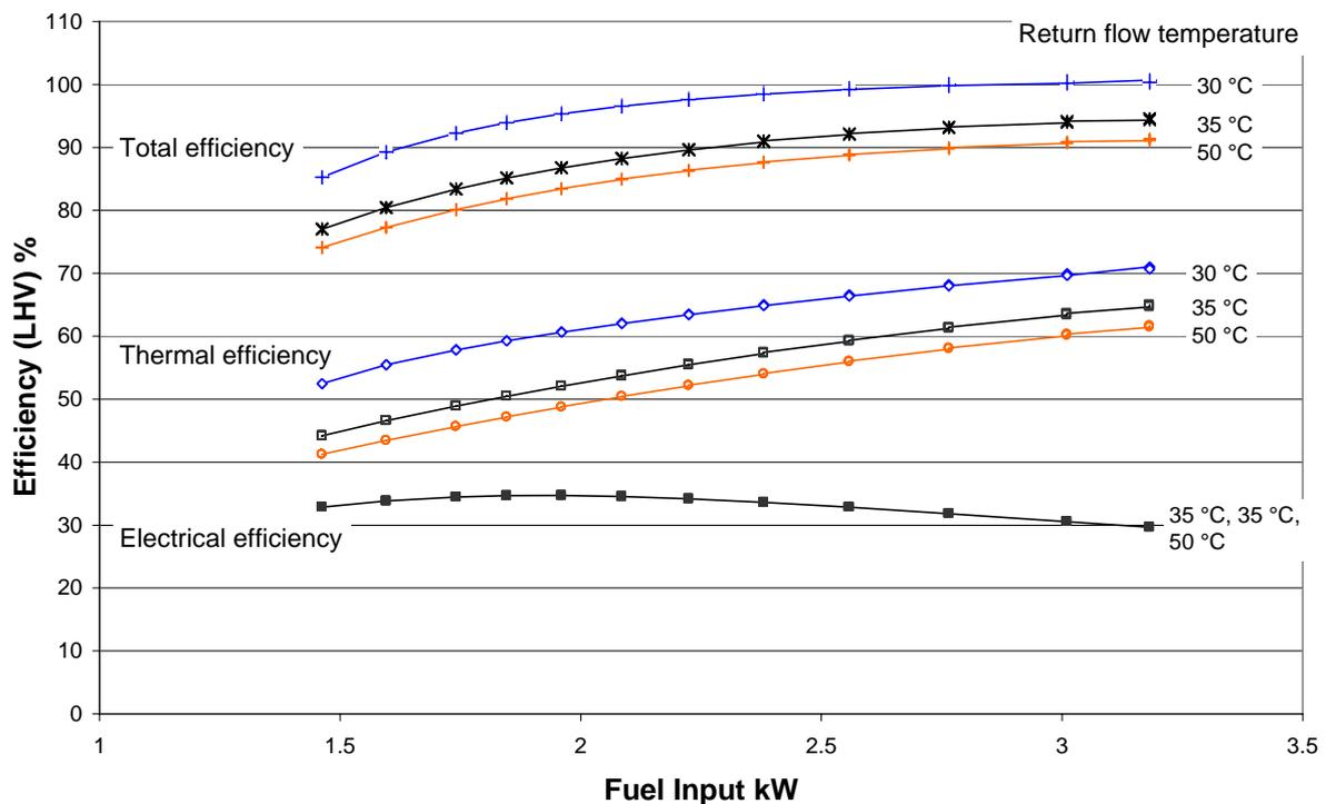
Fig. 6 Electric (AC to grid), thermal and total efficiency performance characteristics of the 1 kW SOFC unit considered, in relation to the power input of the fuel (lower heating value), for three different levels of return flow temperatures
