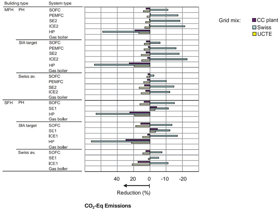
Fig. 27 Reductions of annual CO<sub>2</sub>-eq emissions (%), compared to the GB reference system for the three grid electricity generation mixes considered
