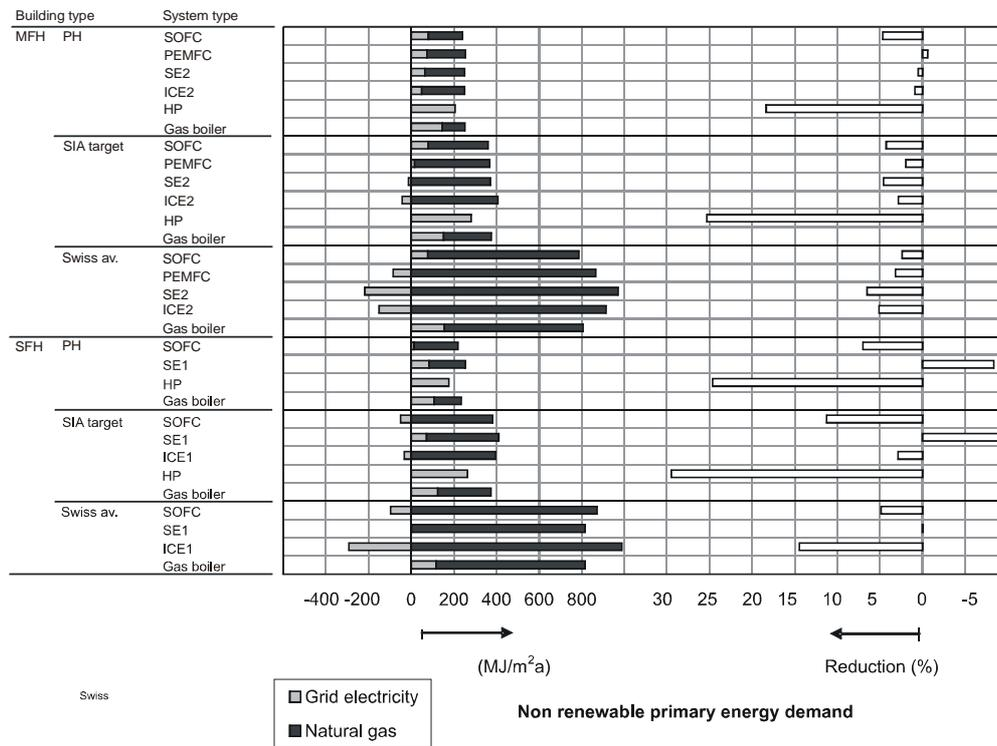
Fig. 17 Annual NRPE demand (MJ/m².a) (for NG and grid electricity) of the basic building and system types analysed, and reductions of NRPE demand (%) compared to the GB reference system “Swiss incl. import” mix.
