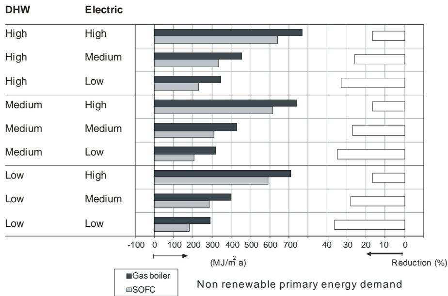
Fig. 40 NRPE demand for the SHF SIA target building equipped with SOFC system for different DHW and electric demand levels, compared to the gas boiler grid reference system. UCTE electricity mix.
