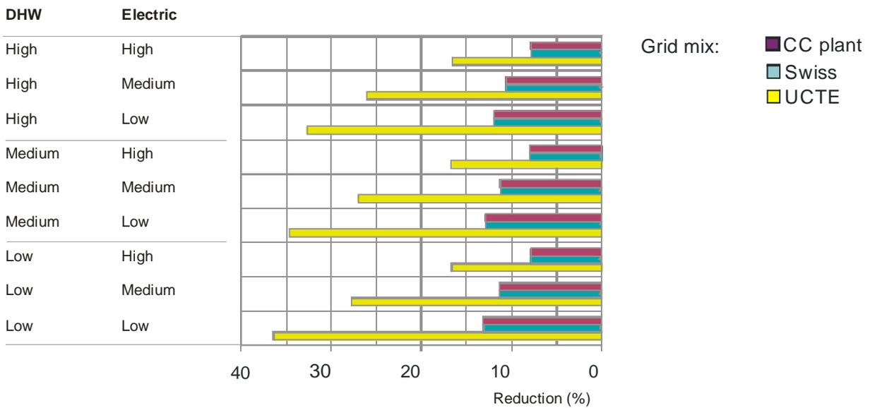
Fig. 41 Relative reductions of NRPE demand for the SHF SIA target building equipped with SOFC system compared to the gas boiler grid reference system, for different DHW and electric demand levels, and for the 3 electricity mixes.
