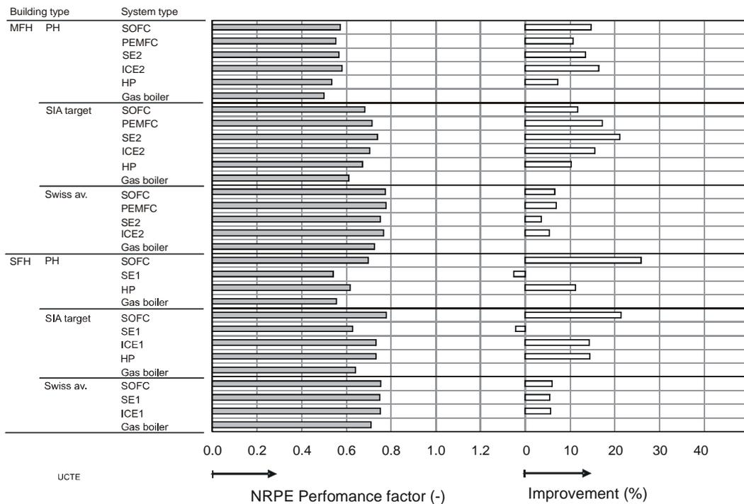
Fig. 20 NRPE performance factor of the basic building and system types analysed, and improvement compared to the NRPE performance factor of the GB reference system (%). UCTE mix
