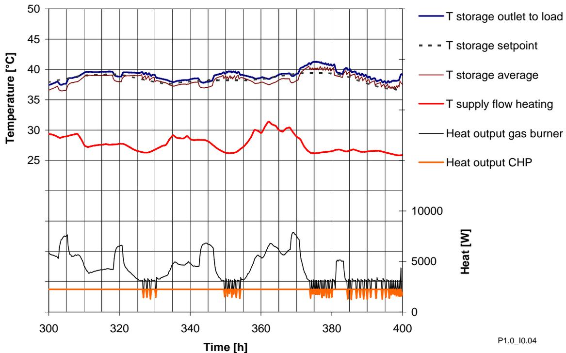
Fig. 44 Influence of PI controller parameters on the storage temperatures and the heat output of the SOFC unit and the auxiliary gas burner. Parameters tuned to optimize the accordance of actual and set point value ( $K_p=2095$ ,  $K_i=83.8$ ). (case SFH SIA building with SOFC MCHP unit)
