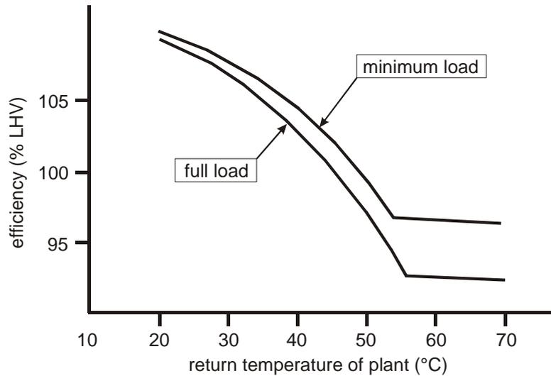
Fig. 11 Efficiency curve of the condensing gas boilers considered
