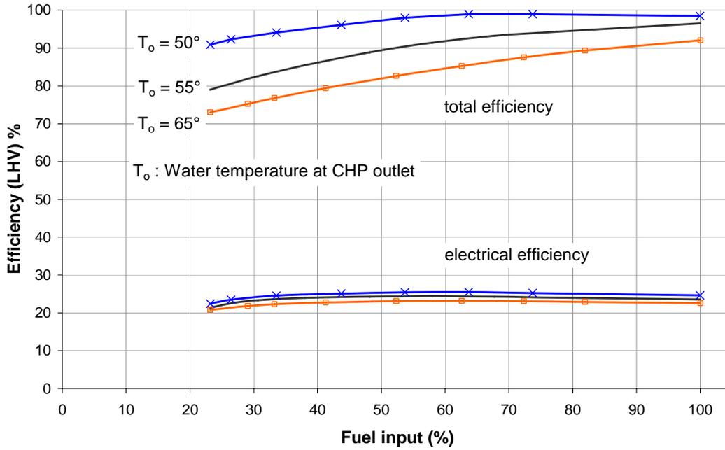
Fig. 9 Electrical and total efficiency performance characteristics of the 9.5 kWe SE unit considered for MFH, for three water temperature levels  $T_o$  for heat supply, at the outlet of the MCHP unit
