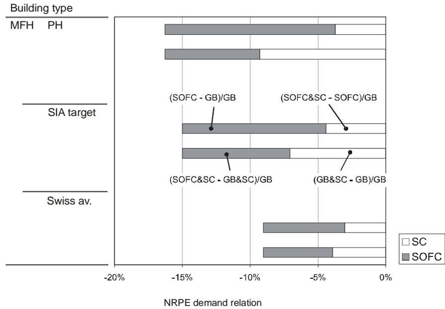
Fig. 29 Comparison of different systems without and with solar collectors (“& SC”), expressed as percentage ratio of NRPE demand of the system, related to the demand standard gas boiler system without solar collector (GB). MFH buildings. UCTE electricity mix.
