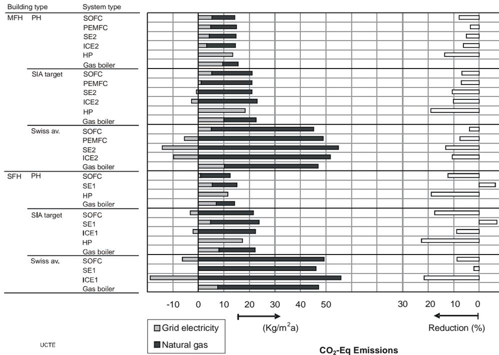
Fig. 24 Annual emissions of  $CO_2\text{-eq}(\text{kg}/\text{m}_2\cdot\text{a})$ (for NG and grid electricity) of the basic building and system types analysed, and reductions of  $CO_{2,\text{equiv}}$  emissions compared to the GB reference system (%). UCTE mix.
