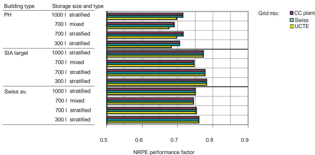
Fig. 39 Influence of storage size on NRPE performance factor for the three electricity generation mixes. SHF building types equipped with SOFC system, for moderate DHW demand profile
