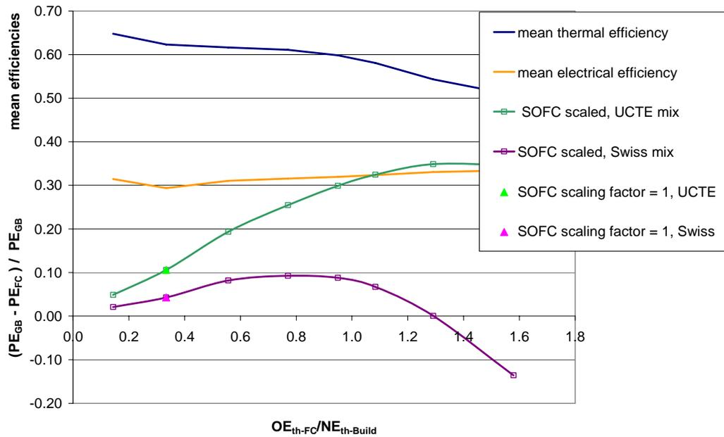
Fig. 36 Difference between NRPE demand of SOFC fuel cell system equipped building ( $PE_{FC}$ ) and NRPE demand of reference building with gas boiler system ( $PE_{GB}$ ), weighted with  $PE_{GB}$ , as a function of the ratio of specific annual thermal output of fuel cell cogen unit ( $OE_{th-FC}$ ) to total annual heat demand of building ( $NE_{th-Build}$ ). Also shown are the resulting mean electrical and thermal efficiencies. Results are given for the UCTE and the Swiss electricity mix.
