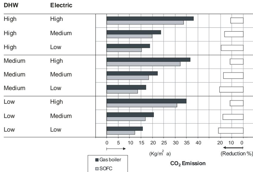
Fig. 42  $CO_2$ -eq emission for the SHF SIA target building equipped with SOFC system for different DHW and electric demand levels, compared to the gas boiler grid reference system. UCTE electricity mix.
