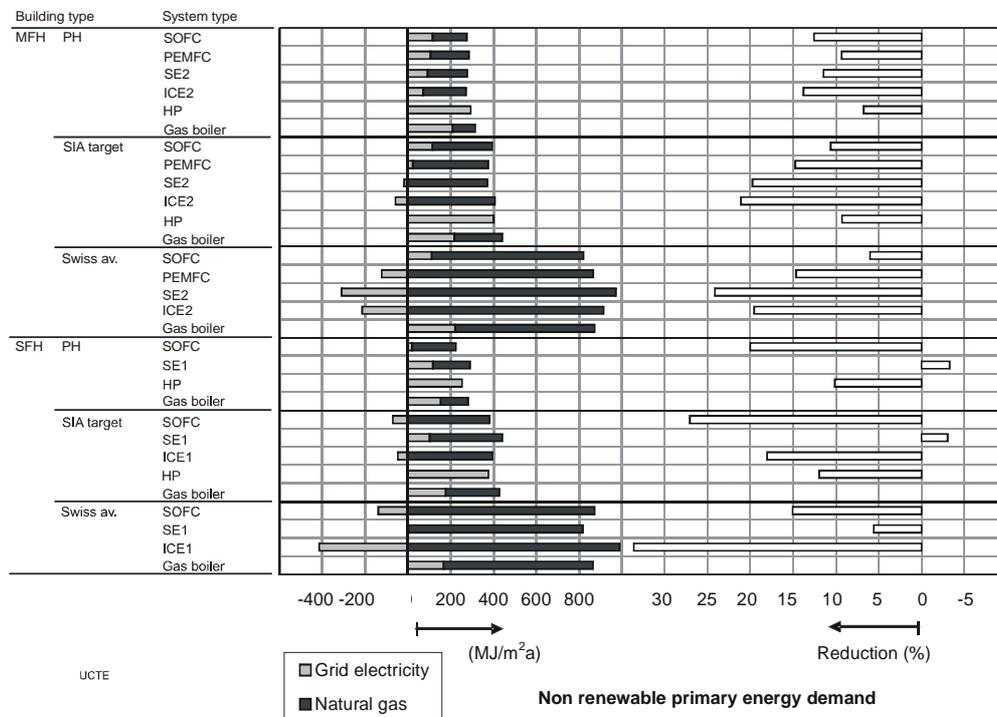
Fig. 16 Annual NRPE demand (MJ/m².a) (for NG and grid electricity) of the basic building and system types analysed, and reductions of NRPE demand (%) compared to the GB reference system. UCTE mix
