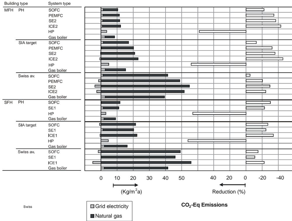
Fig. 25 Annual emissions of  $CO_{2,equiv}$  ( $kg/m^2.a$ ) (for NG and grid electricity) of the basic building and system types analysed, and reductions of  $CO_{2,equiv}$  emissions compared to the GB reference system (%).
