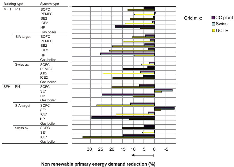
Fig. 19 Reductions of annual NRPE demand compared to the GB reference system for the three grid electricity generation mixes considered
