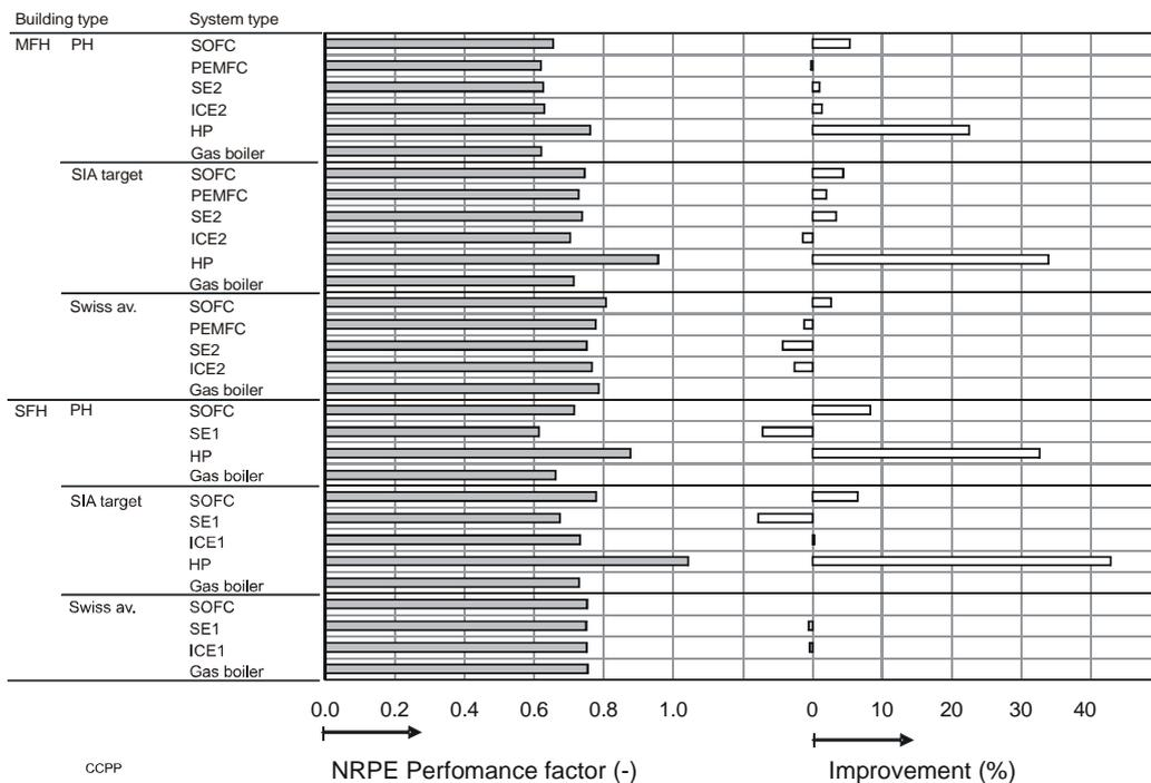
Fig. 22 NRPE performance factor of the basic building and system types analysed, and improvement compared to the NRPE performance factor of the GB reference system (%) “CC power plant” mix
