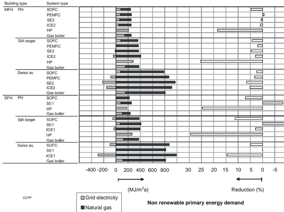
Fig. 18 Annual NRPE demand (MJ/m<sup>2</sup>.a) (for NG and grid electricity) of the basic building and system types analysed, and reductions of NRPE demand (%) compared to the GB reference system. “CC power plant” mix
