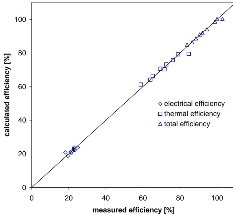
Fig. 7 Goodness of fit between efficiencies derived from measured data and those calculated with the model prior to the assumed improvement of the electrical efficiency
