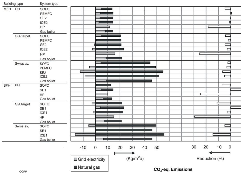
Fig. 26 Annual emissions of  $CO_{2-eq}$  ( $kg/m^2.a$ ) (for NG and grid electricity) of the basic building and system types analysed, and reductions of  $CO_{2-eq}$  emissions compared to the GB reference system (%).
