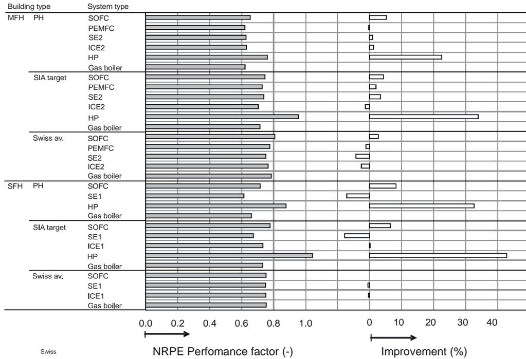
Fig. 21 NRPE performance factor of the basic building and system types analysed, and improvement compared to the NRPE performance factor of the GB reference system (%) “Swiss incl. import” mix
