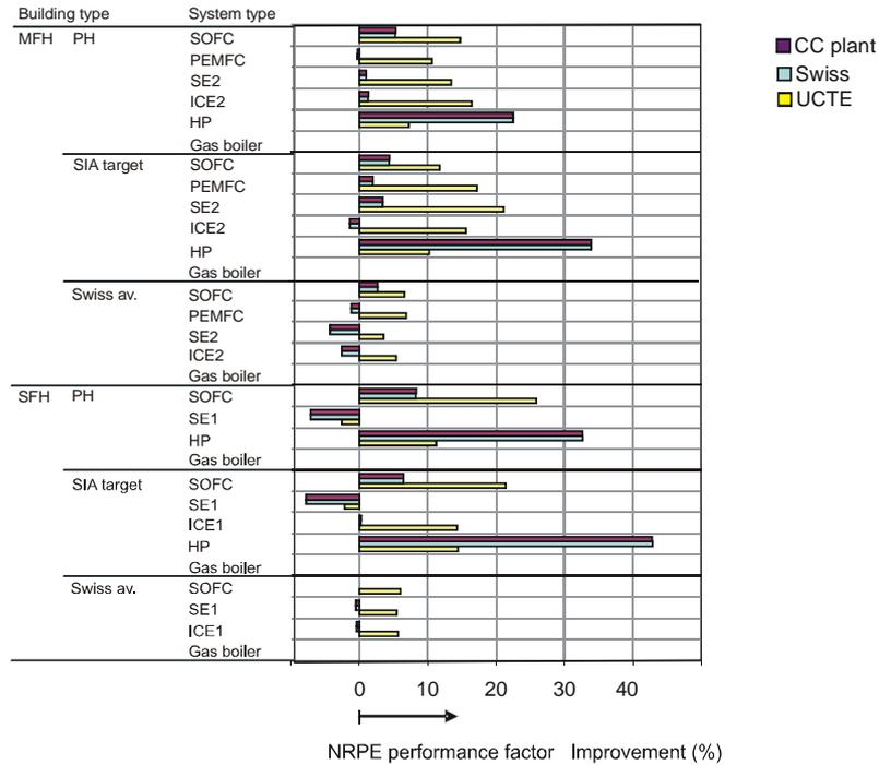
Fig. 23 Improvement of the NRPE performance factor, compared to the GB reference system for the three grid electricity generation mixes considered
