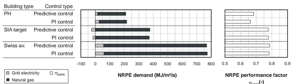
Fig. 46 Non-renewable primary energy (NRPE) demand and NRPE energy performance factor for SFH equipped with SOFC system with optimal predictive and PI control (results from an earlier study (Dorer et al.2005)).
