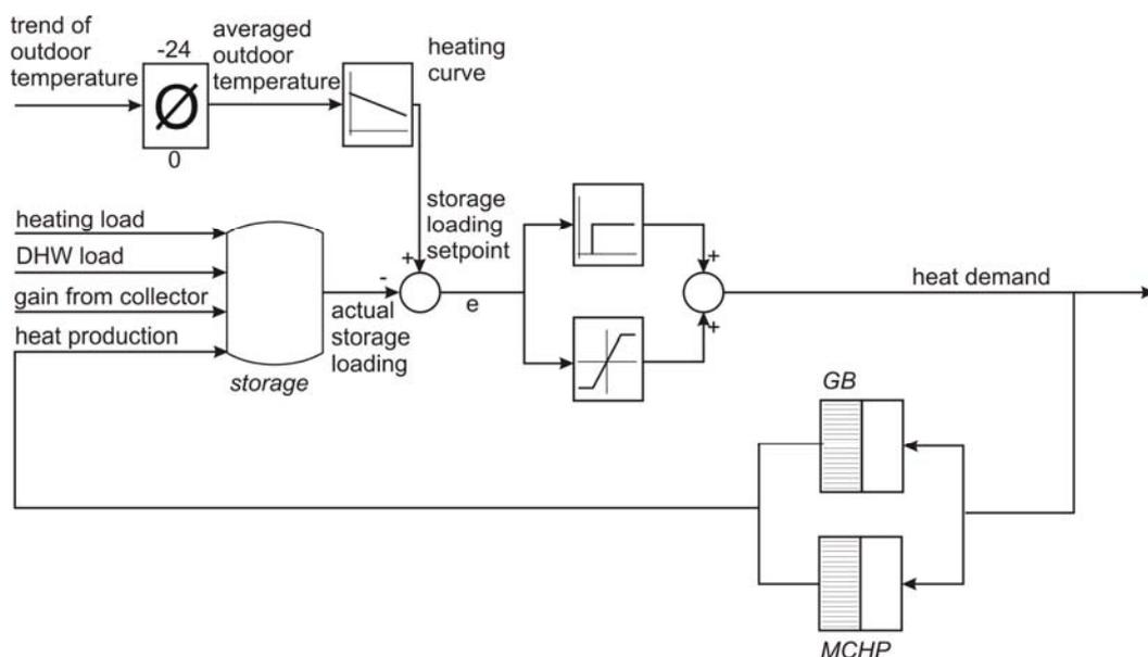
Fig. 14 Schematic of the PI-control of the heat storage temperature
