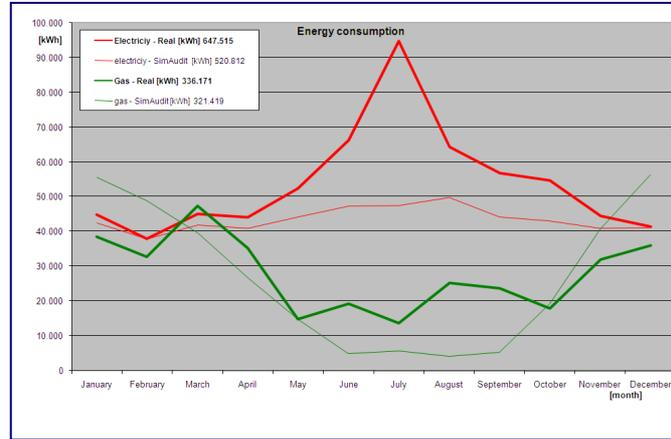
Comparison between the simulated energy consumptions (thin lines) and the measured ones (thick lines). Gas is red, electricity is green.
