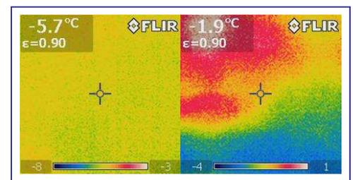
Before defrosting During defrosting Thermographic pictures of the thermosiphon
