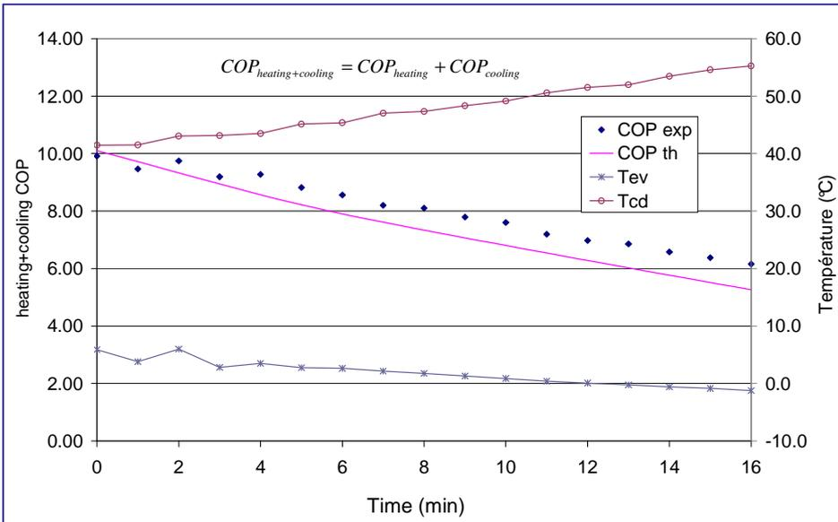
Experimental COP in simultaneous mode compared to compressor selection software values
