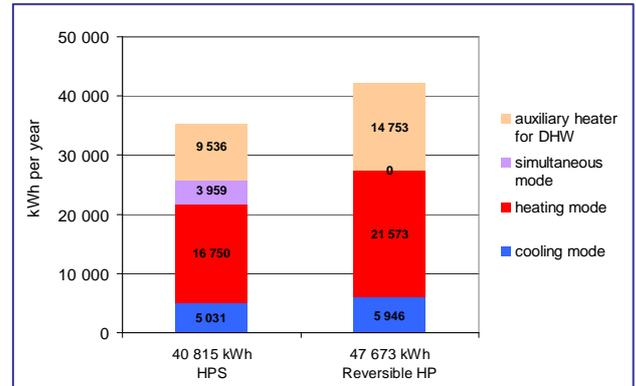
*Electric energy consumption of a HPS and a standard reversible heat pump installed in a 45 bedroom hotel located in Rennes*
