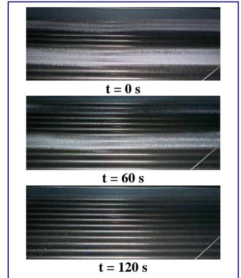
The thermosiphon defrosting sequence lasts 120 s. When the HPS is stopped after a frosting phase, defrosting by the ambient air lasts 20 minutes
