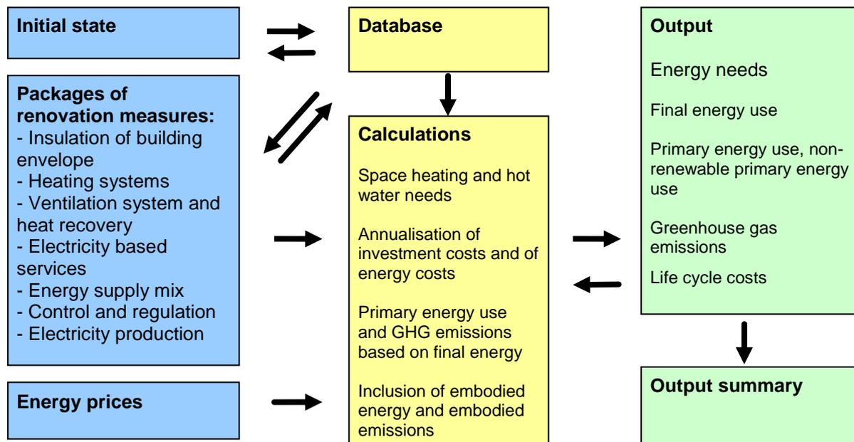
Figure 8 Schematic structure of the INSPIRE tool. The input section is shown in blue; the calculation section is shown in yellow; the output section is shown in green. In the input section and the output section, different boxes represent different worksheets in the Excel-based tool. The calculation section is not visible as such in the tool.
