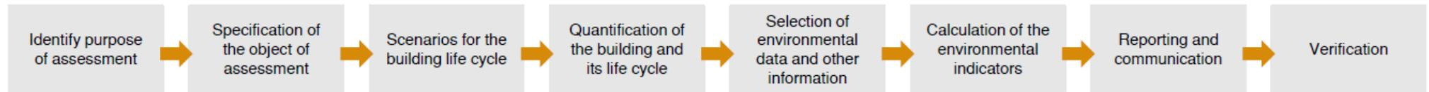
**FIGURE 3:** Illustration of assessment process (as defined in EN 15978:2011)
