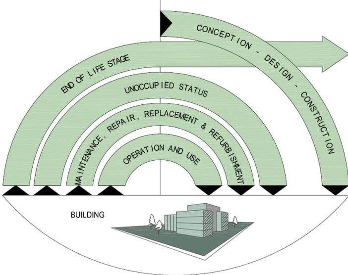
**Figure 1-9:** Model for describing a buildings’ life cycle (adapted from the German Facility Management Association GEFMA (GEFMA, 2004).
