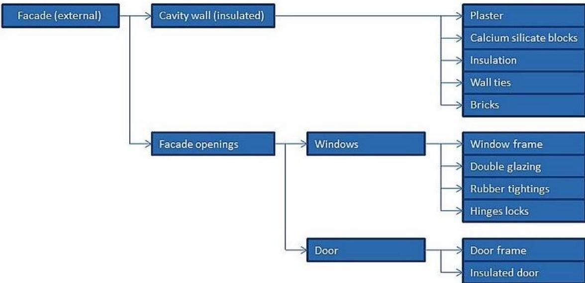
**Figure 1-8:** Example of a structuring of building information using the different level of aggregation specifically for foundation, frame wall and facade (EN 15978:2011).
