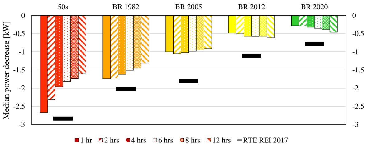
Figure 4.6 Median power decrease in a typical single-family house of 105 m<sup>2</sup> for different modulation durations (medium thermal mass).
